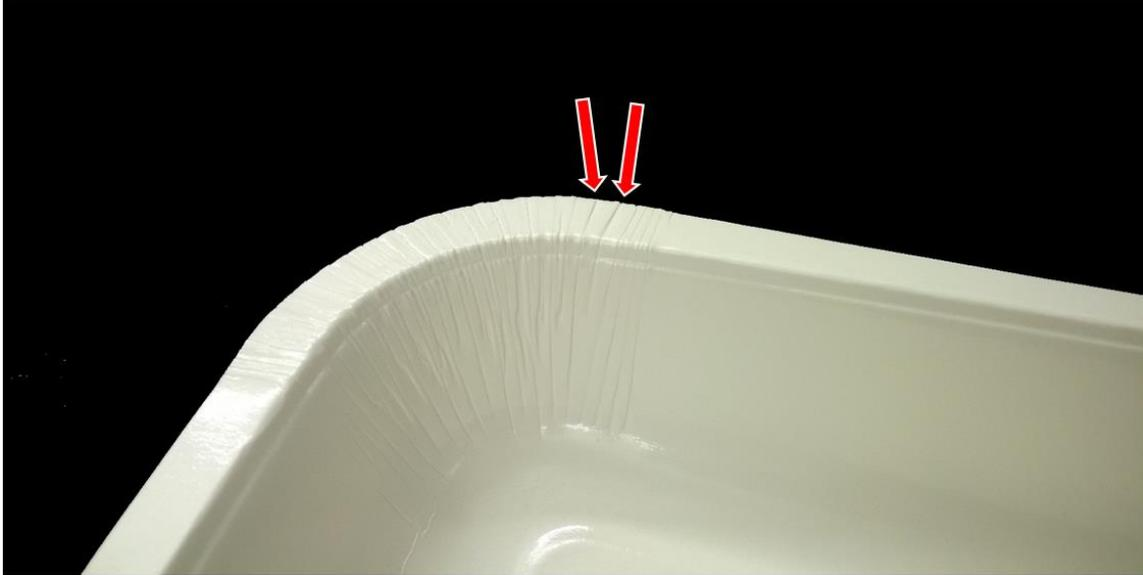
**Fig. 7.** Discarded creases in the tray flange. Creases have not been formed adequately leaving a gap between flat areas surrounding the crease.
