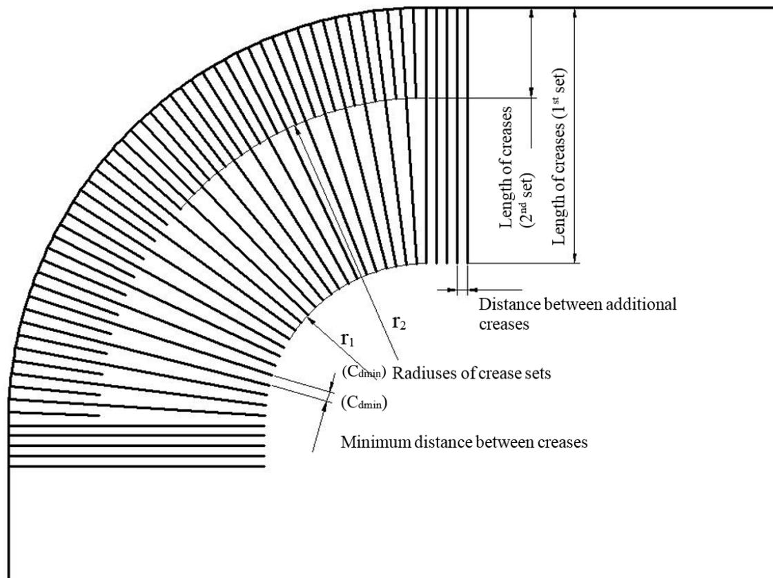
**Fig. 6.** The composition and essential dimensions of creasing
