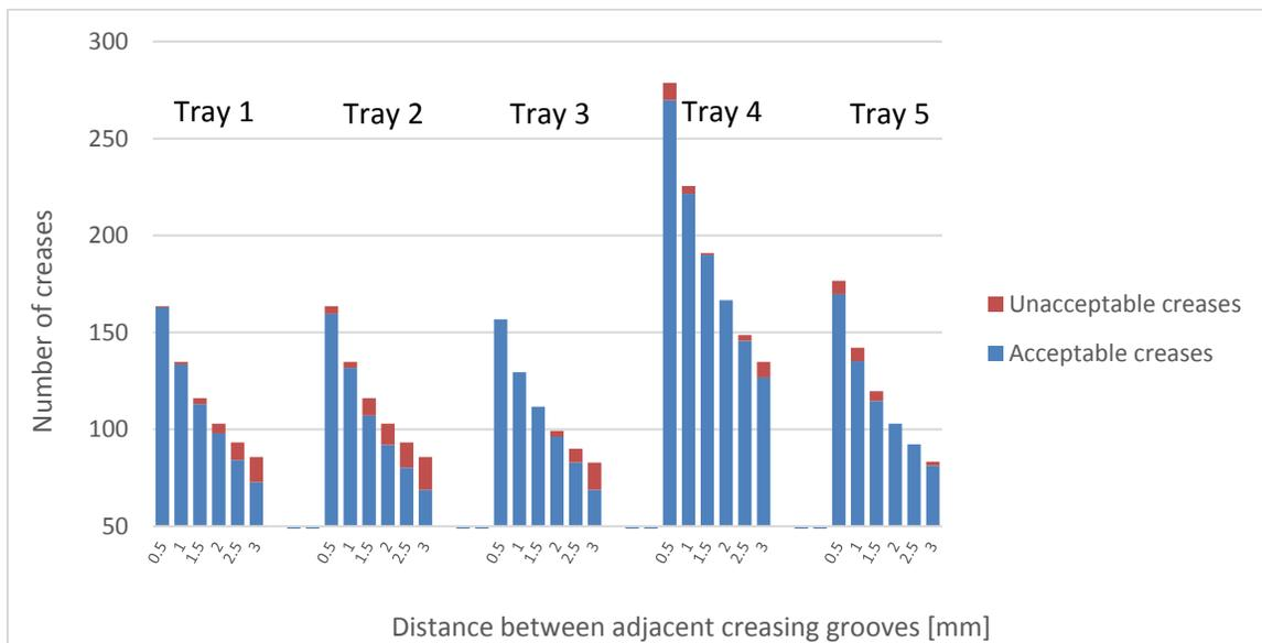
**Fig. 8.** Functionality of creases in test trays
