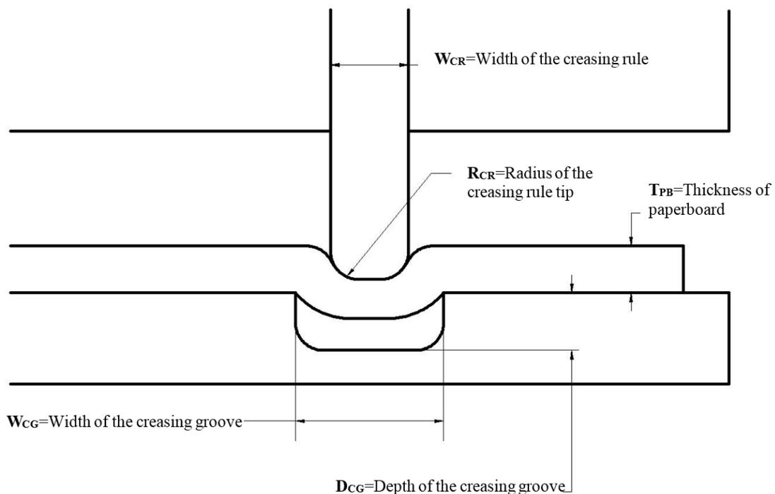
**Fig. 4.** The main dimensions of the creasing rule and groove
