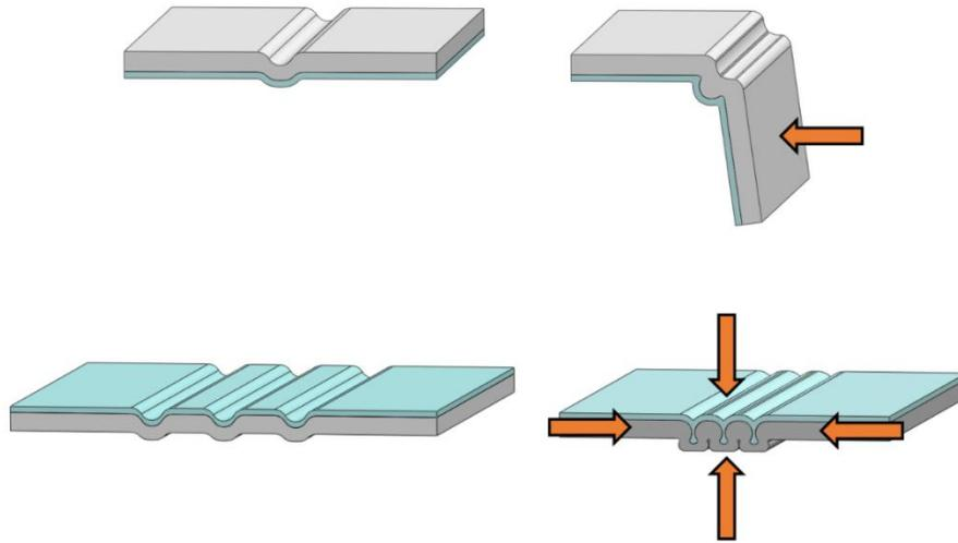
**Fig. 1.** The behavior of creases in folding (above) and in press forming (below). In these methods, creasing is performed on different sides of the substrate to retain the polymer barrier layer inside the package.
