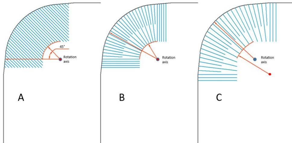
**Fig. 3.** Creasing pattern designs. A) Creases are positioned in a  $45^\circ$  angle parallel to each other; B) creases are positioned radially toward the rotation axis of the tray corner; C) creases are positioned radially toward a point deviating 10 to 30 mm from the rotation axis of the tray corner.
