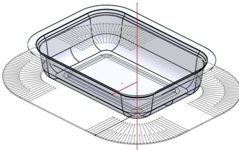
**Fig. 2.** A paperboard blank and the final product of the tray pressing process. The folding of the paperboard blank is controlled with creases in addition to actual forming parameters. The radius and the rotation axis of the tray corner are marked in red.
