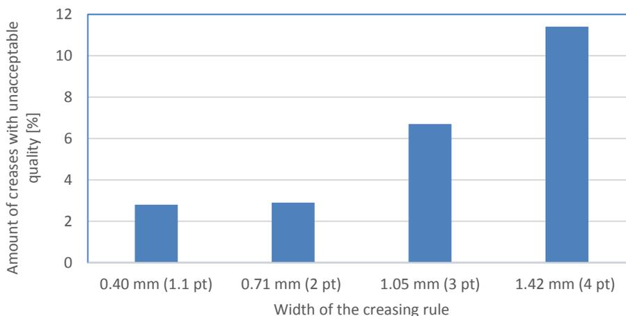
**Fig. 5.** The amount of creases with unacceptable quality resulting from different creasing rule widths. Values are the average of ten trays.
