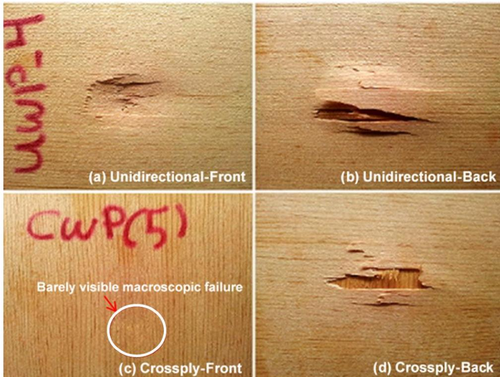
**Fig. 5.** Unidirectional and cross-ply Douglas fir laminates after impact testing: a) unidirectional, front surface; b) unidirectional, back surface, fracture in all layers; c) cross-ply, front surface; and d) cross-ply, back surface, controlled fracture in alternative layers
