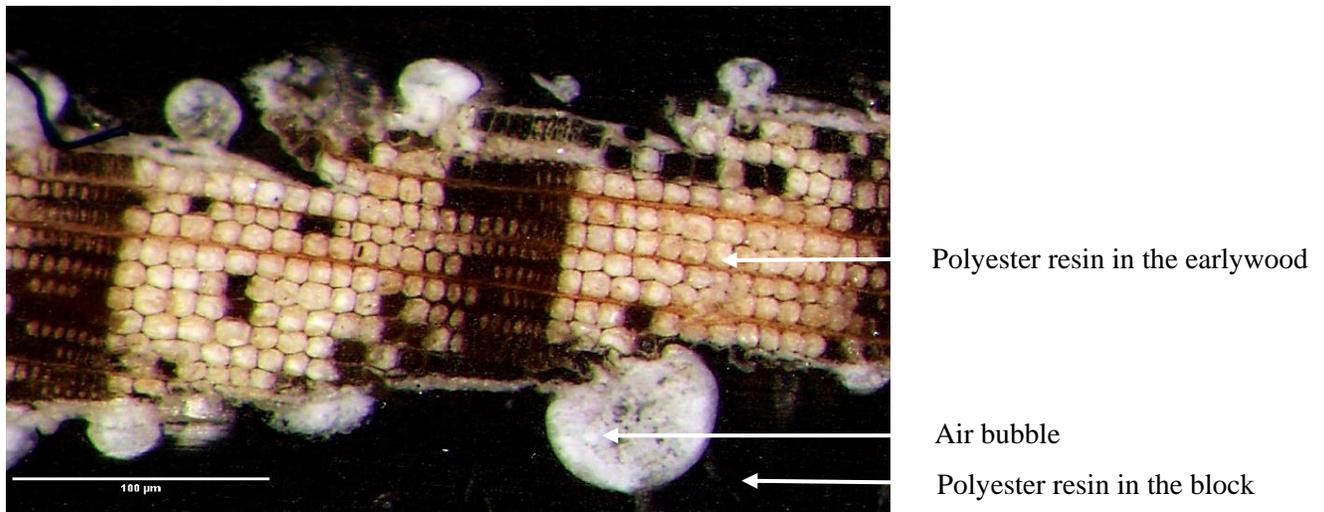
**Fig. 3.** Light micrograph of the resinated veneer sheet in a polyester block
