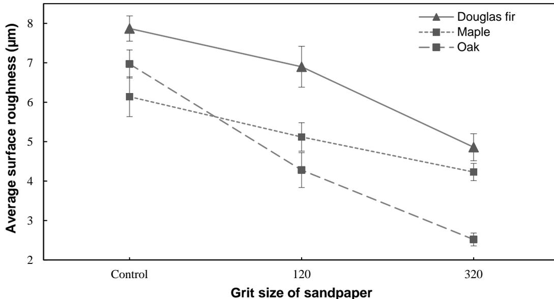
**Fig. 10.** Surface roughness of veneers as a function of sandpaper grit size; Error bars represent 95% confidence intervals.
