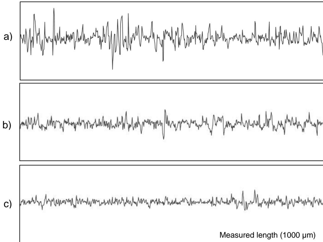
**Fig. 11.** Roughness profiles of the oak veneer before and after sanding: (a) control oak; (b) sanded with grit 120; and (c) sanded with 320-grit sandpaper
