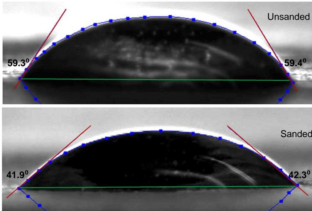
**Fig. 9.** Contact angles of polyester droplets on oak veneer before and after sanding with grit size of 120 (angles at 0.5 second)
