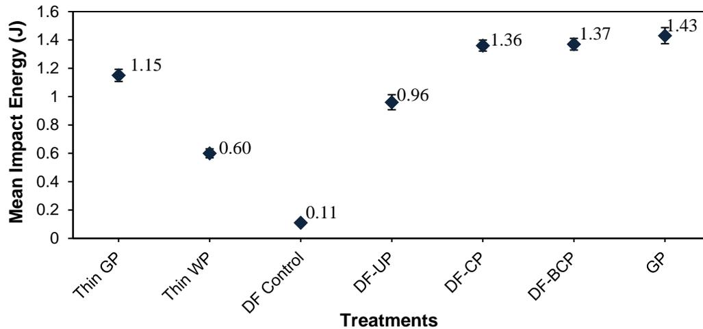
**Fig. 6.** Comparison of the mean impact energy of wood/polyester and glass fiber/polyester composite laminates (error bars represent 95% confidence intervals). Note: Impact energy values of Thin GP and Thin WP were taken from a previous study (Haghdan *et al.* 2015).
