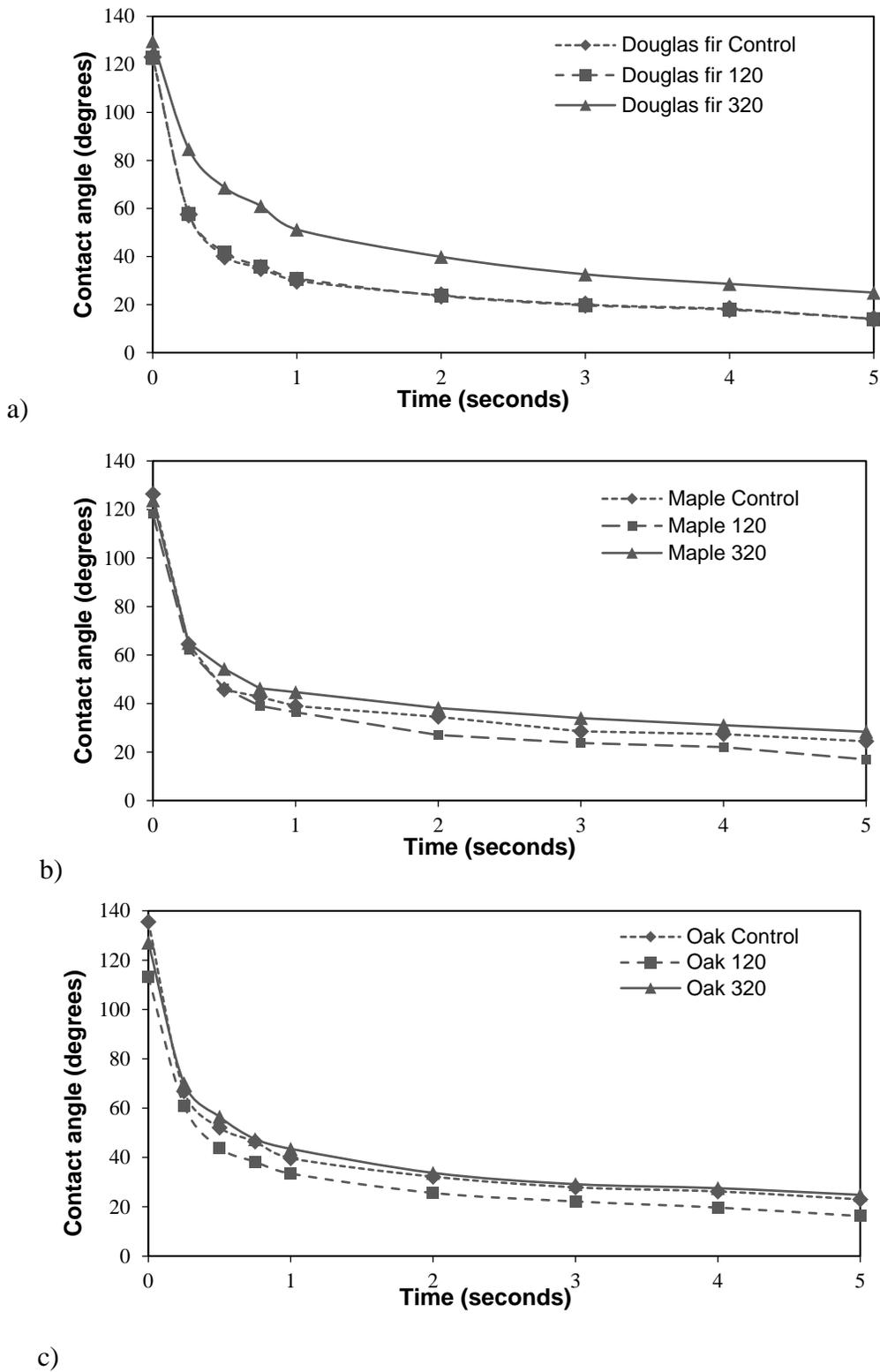
Fig. 8. Contact angle of polyester droplets on wood veneers (before and after sanding) vs. time: a) Douglas fir veneer; b) maple veneer; and c) oak veneer
