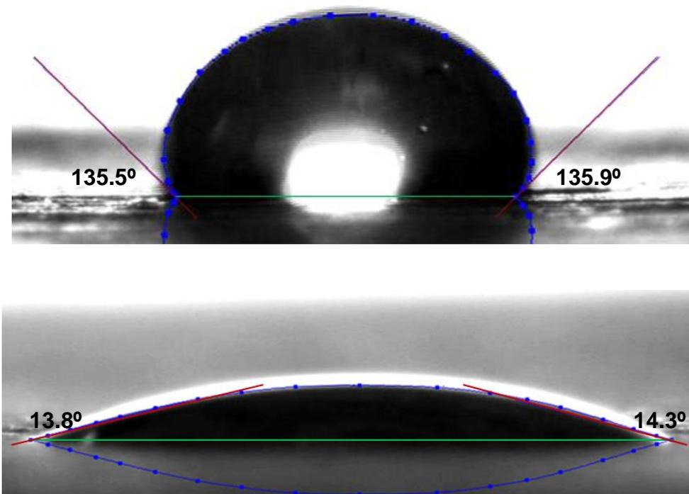
**Fig. 7.** Highest initial angle of polyester droplet on Oak Control (top), and lowest angle of polyester droplet after 5 s, DF 120 (bottom)
