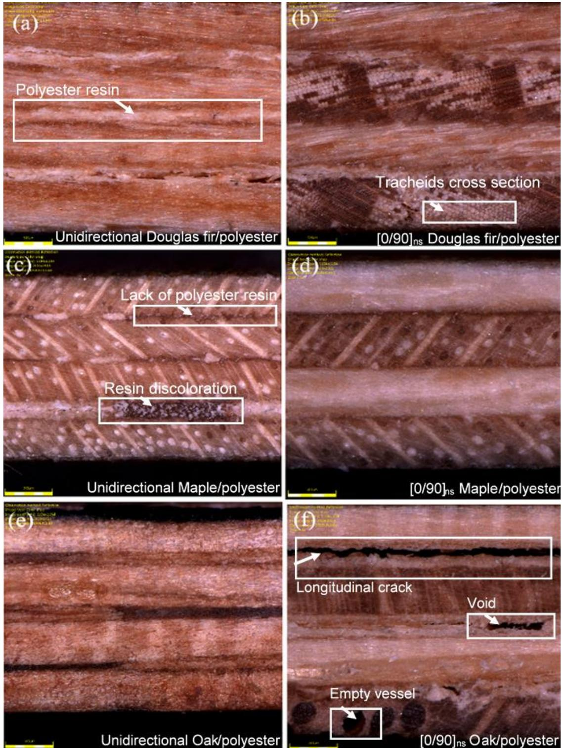
**Fig. 4.** Light microscopic images of unidirectional and cross-ply polyester laminates: (a) polyester as a white strip between layers; (b) filled cross sections of longitudinal tracheids with resin; (c) resin discoloration and area of lack of polyester; (d) neat adhesion among layers; (e) insufficient adhesion and voids; and (f) crack, void, and vessel elements
