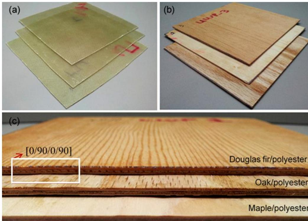
**Fig. 2.** Composite laminates after curing (a) glass fiber/polyester, (b) unidirectional wood/polyester, and (c) cross-ply wood/polyester
