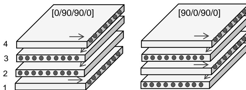
**Fig. 1.** Lay-up of two cross-ply wood composite laminates made of four laminae; balanced (*left*), and unbalanced (*right*); arrows indicate the fiber direction. Resin applied to the top face of the layers one to three is not shown here.
