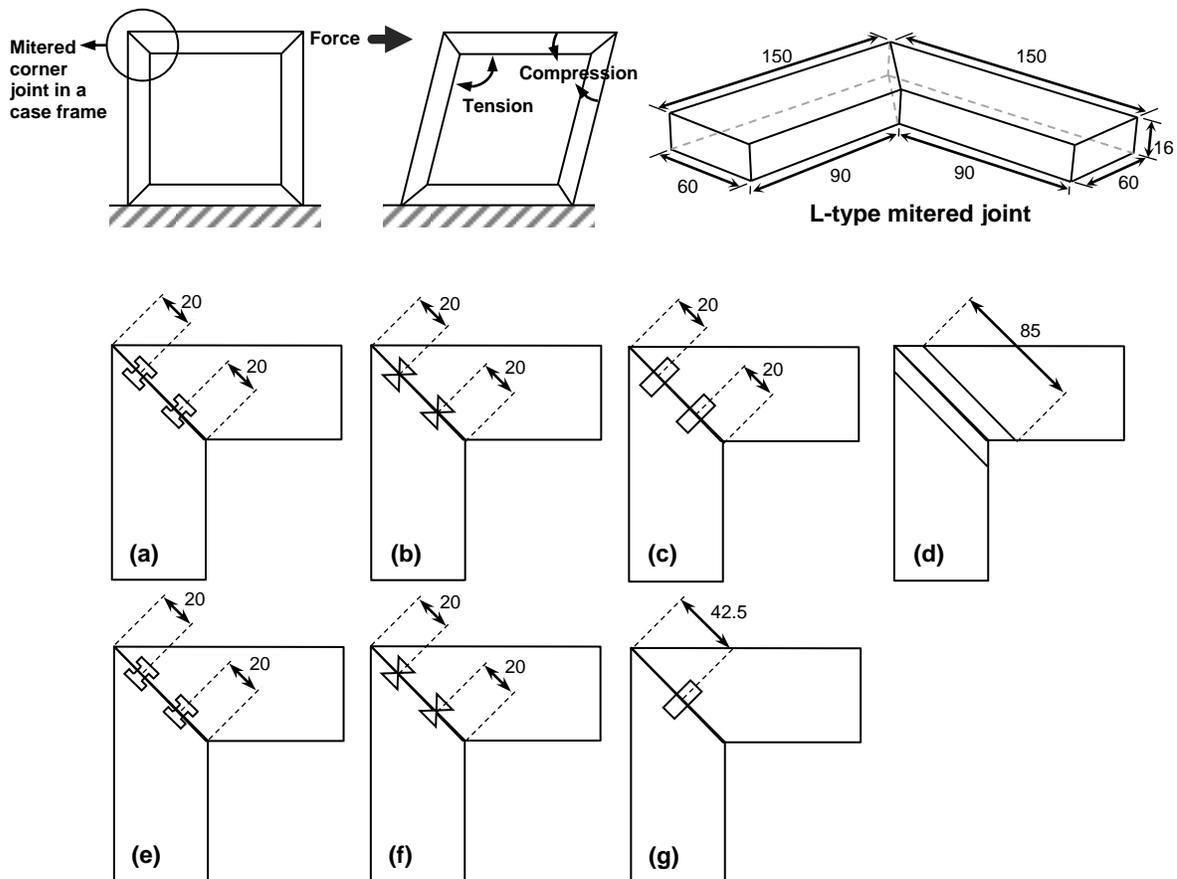
**Fig. 2.** Dimensions (mm) and configurations of L-type mitered joints with different fasteners; (a): glued joint with H-shaped dovetail keys; (b): glued joint with butterfly dovetail keys, (c): two-pin dowel joint; (d): plywood spline joint; (e): unglued joint with H-shaped keys; (f): unglued joint with butterfly keys; (g): one-pin dowel joint
