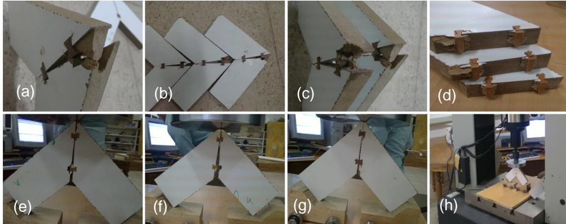
**Fig. 4.** Examples of panel failures in joints with dovetail keys; (a), (b), and (c) are glued mitered joints with dovetail keys tested in compression; (d), (e), (f), (g), and (h) are glued mitered joints with dovetail keys tested in tension
