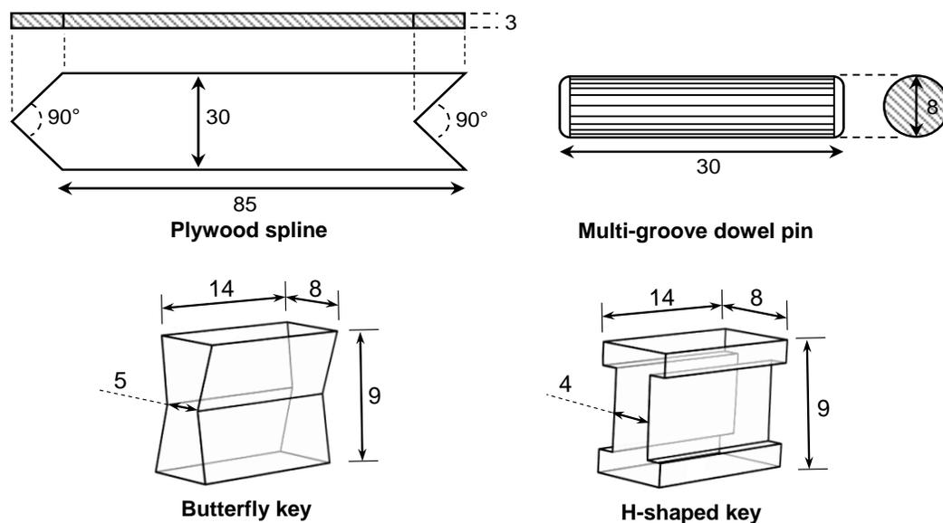
**Fig. 1.** Geometry of fasteners used in the study (measurements in mm)
