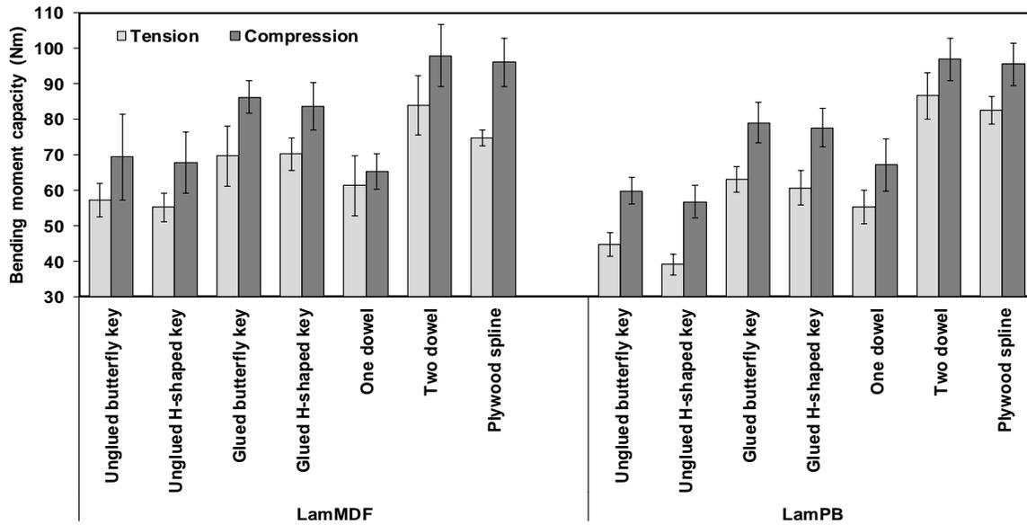
**Fig. 5.** Bending moment capacity of Laminated MDF and Laminated PB joints as a function of joint type
