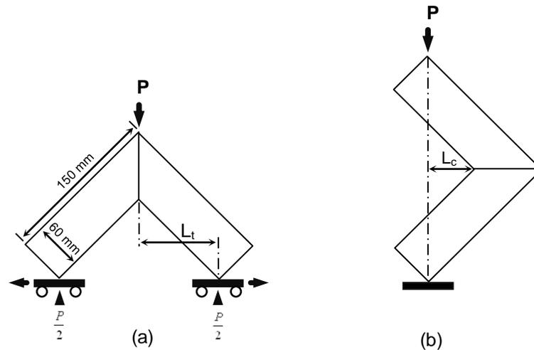
**Fig. 3.** Method of loading of L-shaped joints specimens; (a): tension test, (b): compression test
