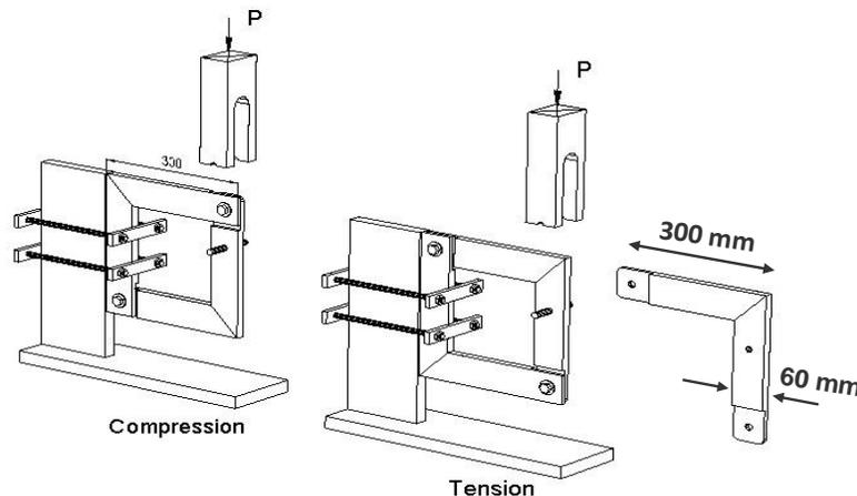
**Fig. 6.** Loading form of the 300 mm square frame specimens constructed with two-pin dowel joints
