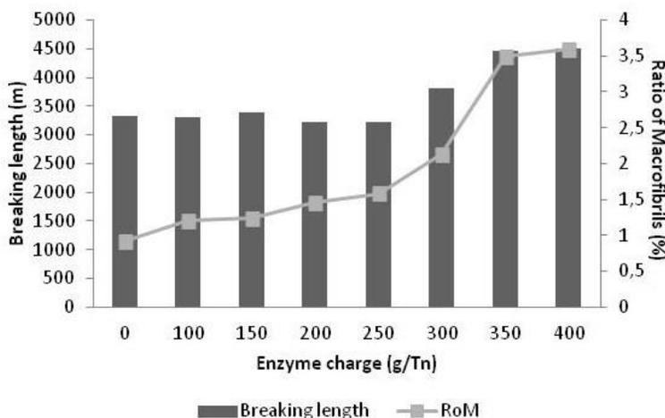
Fig. 2. Effect of enzyme charge on paper breaking length and RoM
