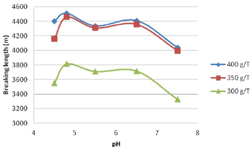
Fig. 4. Effect of pH in biorefining treatments
