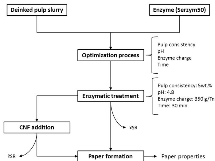
Fig. 1. Experimental procedure of the present work
