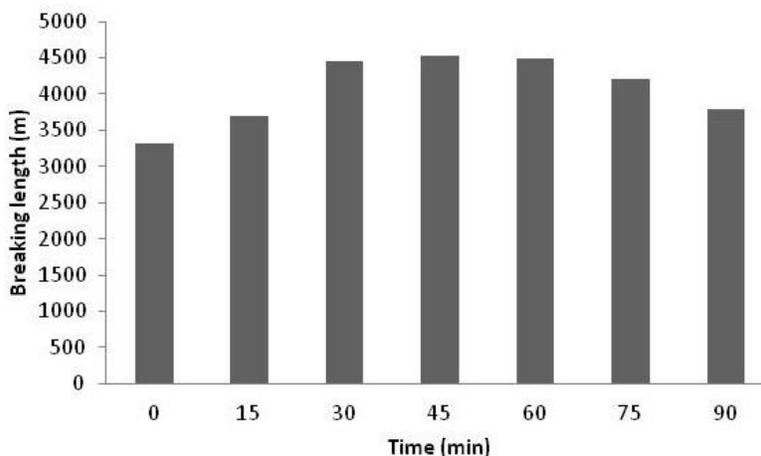
**Fig. 6.** Effect of reaction time on paper breaking length
