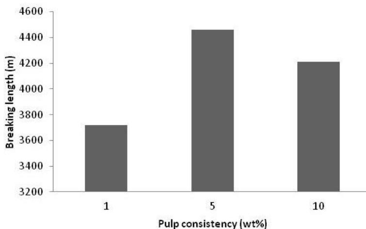
Fig. 5. Effect of pulp consistency on paper breaking length
