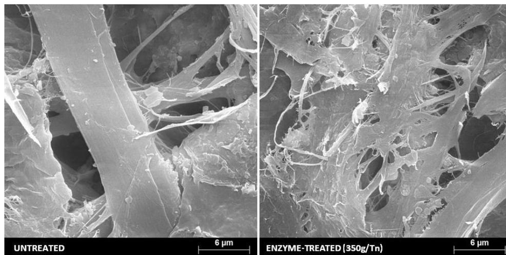
**Fig. 7.** SEM images of untreated and enzyme-treated paper sheets
