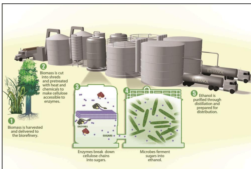
Fig. 1. Schematic of an example of cellulosic ethanol production process (Office of Biological and Environmental Research of the U.S. Department of Energy Office of Science)
