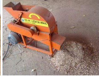
Fig. 7. The GXP-400 crumbling machine
