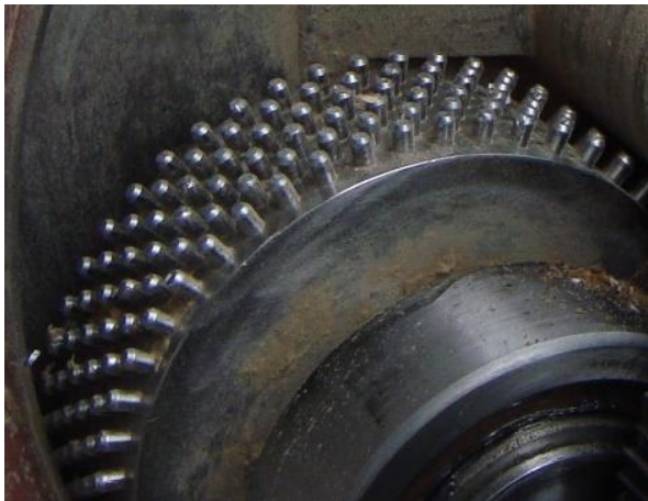
Fig. 13. The surface of the roller after work
