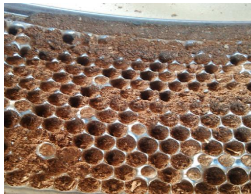
Fig. 5. Ring die failure with wear and deformation
