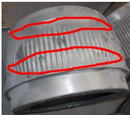
Fig. 4. Roller failure with wear
