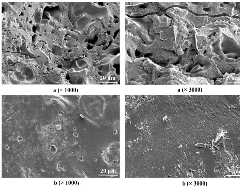
**Fig. 6.** MUF resin: a) formulation A1 b) formulation A3
