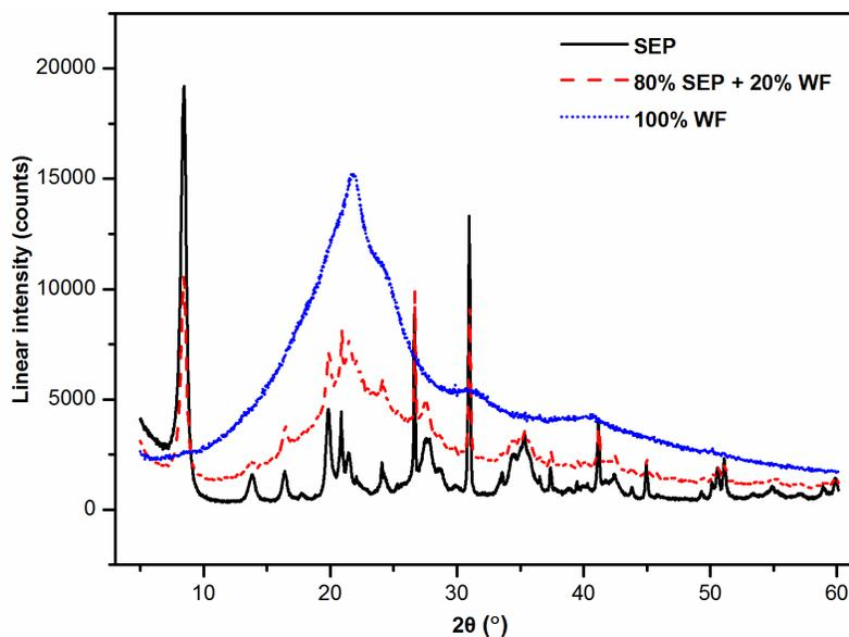
**Fig. 2.** XRD patterns of the SEP and MUF resin with various filler formulations: (A1) 100% WF and (A3) 80% SEP + 20% WF
