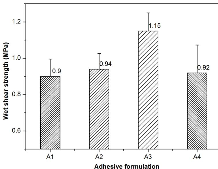
**Fig. 3.** The wet shear strength of plywood bonded by MUF resin with various filler formulations: (A1) 100% WF, (A2) 40% SEP + 60% WF, (A3) 80% SEP + 20% WF, and (A4) 100% SEP
