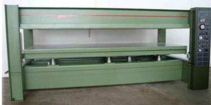
Fig. 2. Hydraulic pressing machine model UT6L
