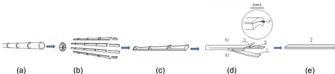
**Fig. 1.** Sketch of the sample processing: (a) raw bamboo; (b) radial splitting; (c) bamboo strips; (d) tangential splitting; (e) bamboo sliver; 1) near the bamboo inner skin; 2) near the bamboo outer skin; 3) outer skin; A-A) Cross section; F) Cutting face
