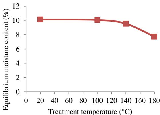
**Fig. 2.** Equilibrium moisture content of bamboo before and after heat treatment
