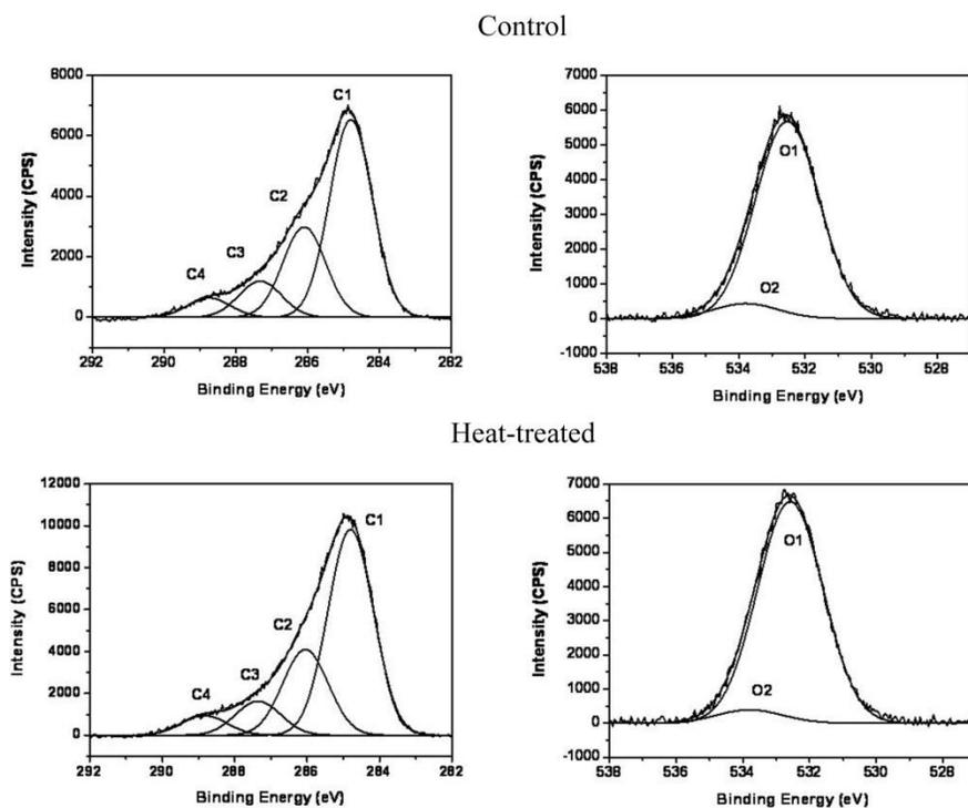
Fig. 3. C<sub>1s</sub> and O<sub>1s</sub> XPS survey spectra of control and heat-treated samples
