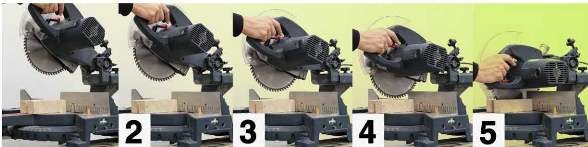
Fig. 2. Sequential saw blade movement through the sample with manual feeding
