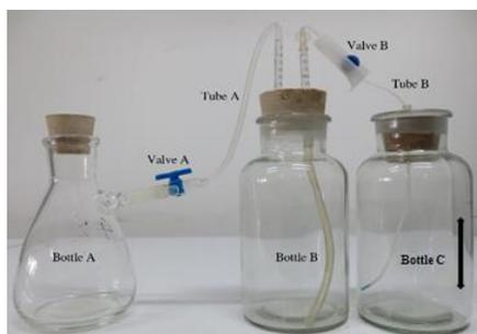
**Fig. 1.** Lab-scale setup for anaerobic digestion. Bottle A: anaerobic reactor; Bottle B: biogas collector; Bottle C: solution collector; Tube A: biogas-guide tube; Tube B: solution-guide tube; Valve A was used for biogas sampling; Valve B for biogas metering.
