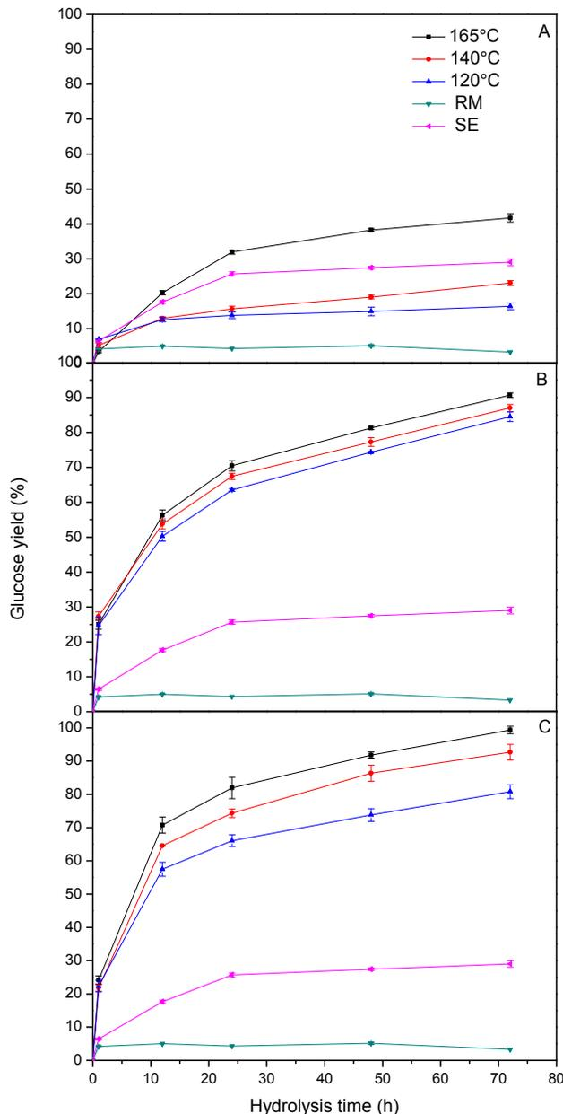
**Fig. 3.** Comparison of enzymatic hydrolysis profiles of the AS (A), AL (B), and ALS (C) pretreated bamboo
