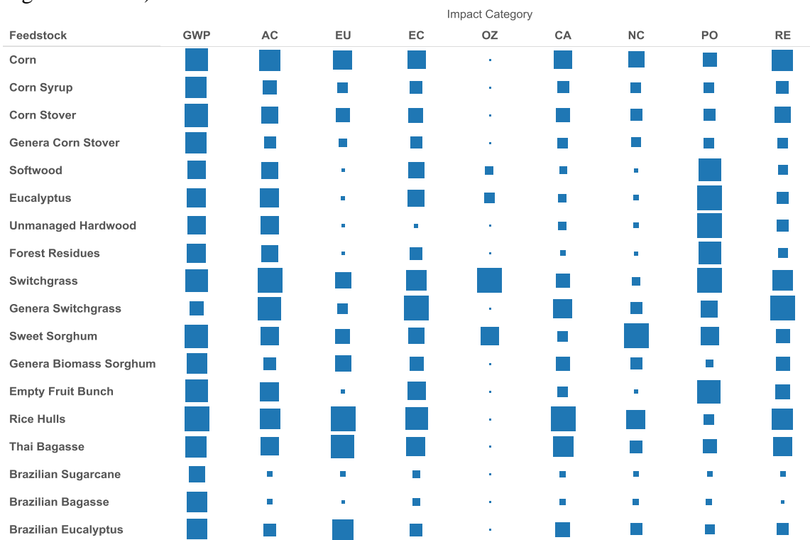
Fig. 5. TRACI impact assessment results for all feedstocks cradle-to-gate. Larger squares indicate higher environmental impact within a category per BDMT. Raw TRACI impact values in table form can be found in Appendix Table A2. For the GWP impact category all of the scenario values were negative; in this plot the size of the square is larger for those scenarios with larger net GWP impacts.
