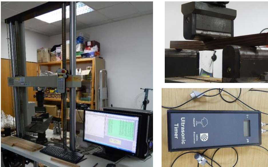
Fig. 5. TIRA 50 kN testing machine (left), a rupture of heat-treated wood under the bending load (top right), and Fakopp Ultrasonic Timer instrument (bottom right)
