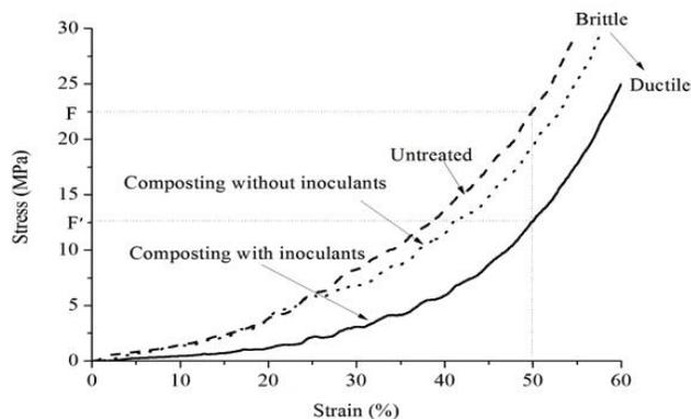
**Fig. 6.** Stress-strain curves of rice husks with and without composting
