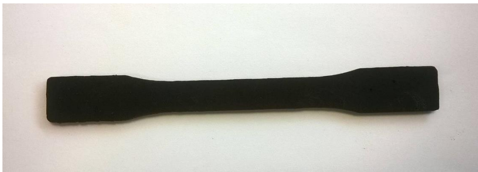
Fig. 2. PU film sample for stress-strain testing
