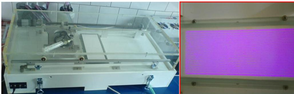
Fig. 2. DCSBD plasma generator and electrodes covered by plasma (in air)
