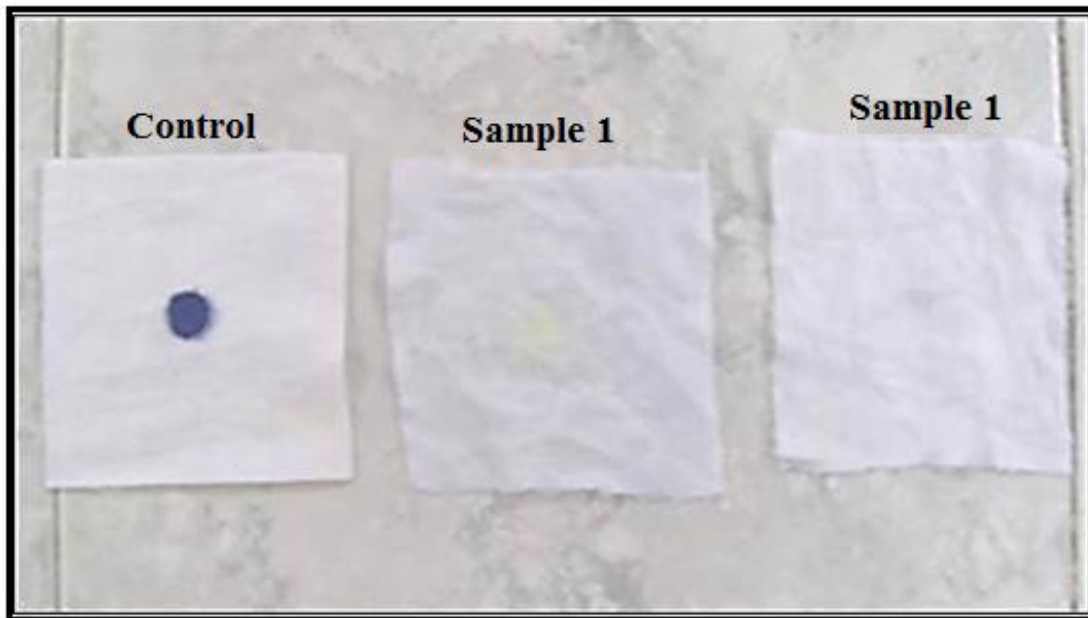
Fig. 7. De-staining ability of purified endoglucanase: Sample 1 was treated with detergent-only solution, presenting yellowish ink stain retained on it, while Sample 2 was treated with detergent solution with the addition of purified endoglucanase enzyme, displaying the complete elimination of the ink stain as compared with the control sample.
