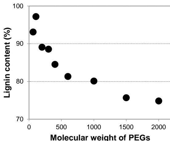
**Fig. 1.** Effect of PEG molecular weight on the lignin content of alkaline PEG-treated lignin prepared from purified lignin
