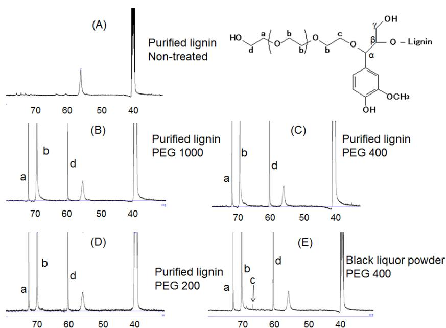
**Fig. 5.**  $^{13}\text{C}$ -NMR spectra of (A) purified lignin, alkaline PEG-treated lignin prepared from (B) purified lignin with PEG 1000, (C) purified lignin with PEG 400, (D) purified lignin with PEG 200, and (E) black liquor powder with PEG 400
