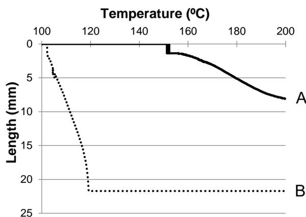
**Fig. 3.** Thermal softening length of alkaline PEG-treated lignin prepared from (A) purified lignin and (B) black liquor powder
