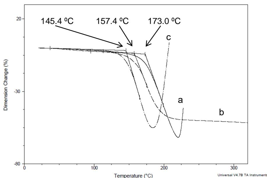
**Fig. 4.** Thermal mechanical analysis of (a) purified lignin; (b) alkaline PEG-treated lignin prepared from black liquor powder; and (c) alkaline PEG-treated lignin prepared from purified lignin
