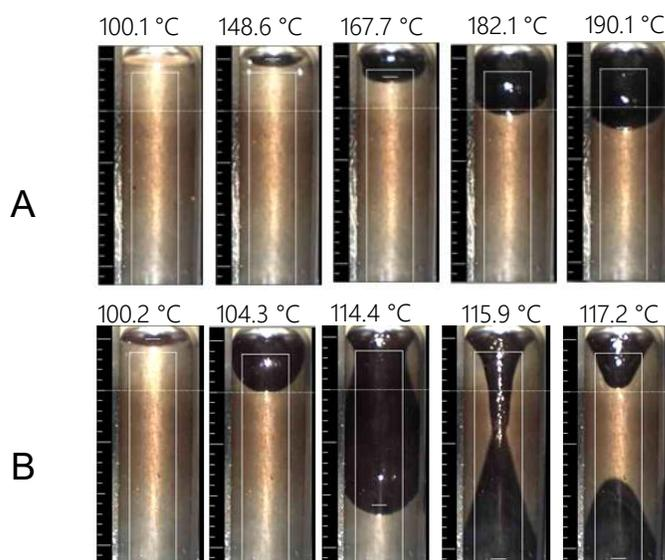
**Fig. 2.** Thermal softening behavior of alkaline PEG-treated lignin prepared from (A) purified lignin and (B) black liquor powder with increasing temperature to determine softening point
