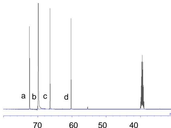
**Fig. 7.**  $^{13}\text{C}$ -NMR spectrum of alkaline PEG-treated lignin prepared from the acid-soluble lignin fraction
