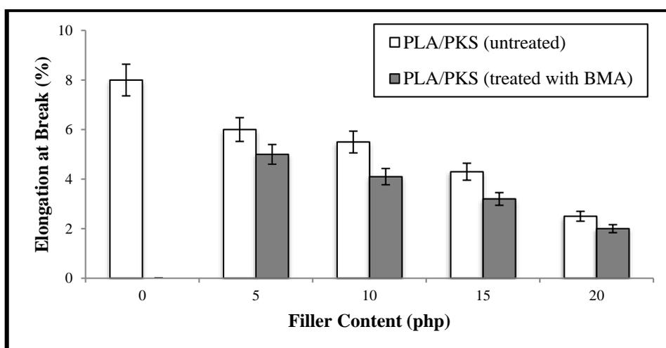
**Fig. 2.** Effect of filler content on the elongation at break of untreated and treated PLA/PKS biocomposite films
