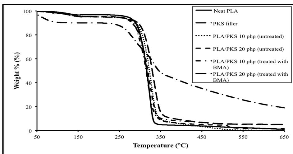
Fig. 8. TGA curve of neat PLA, and untreated and treated PLA/PKS biocomposite films
