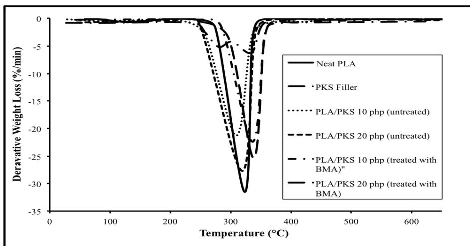
Fig. 9. DTG curve of neat PLA, and untreated and treated PLA/PKS biocomposite films
