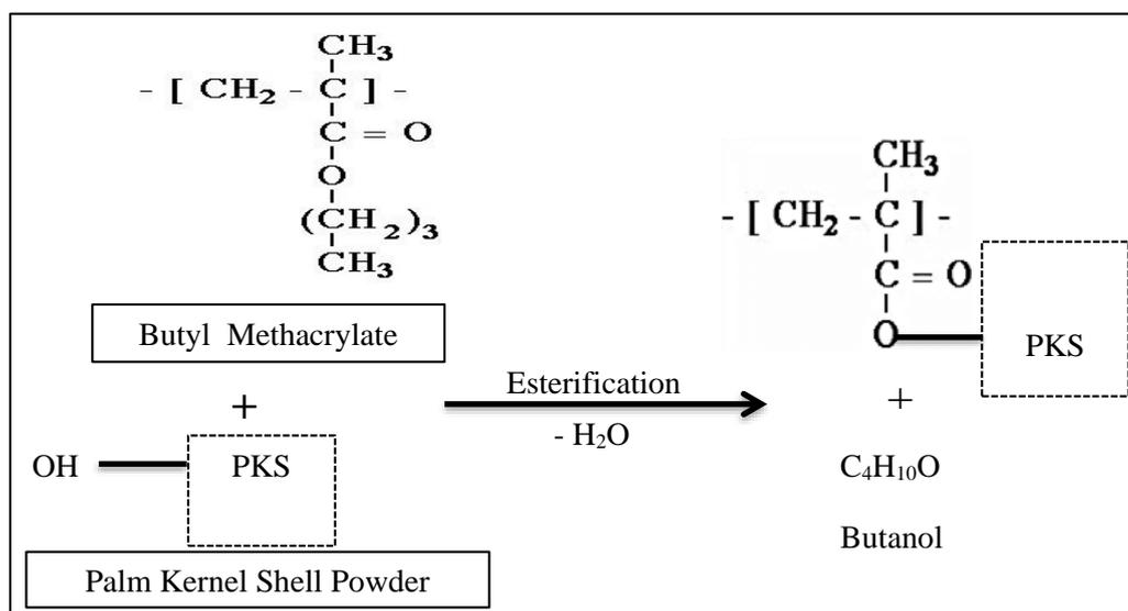
Fig. 7. Schematic reaction of PKS with BMA and PLA
