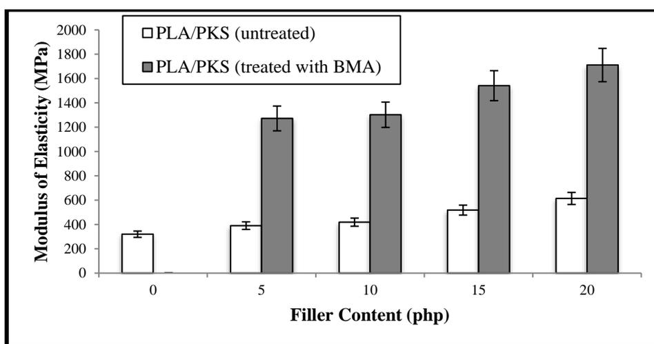
**Fig. 3.** Effect of filler content on the modulus of elasticity of untreated and treated PLA/PKS biocomposite films
