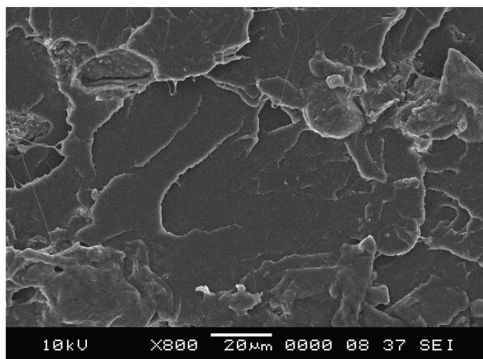
Fig. 5. SEM micrograph of treated PLA/PKS biocomposite film (10 php PKS)
