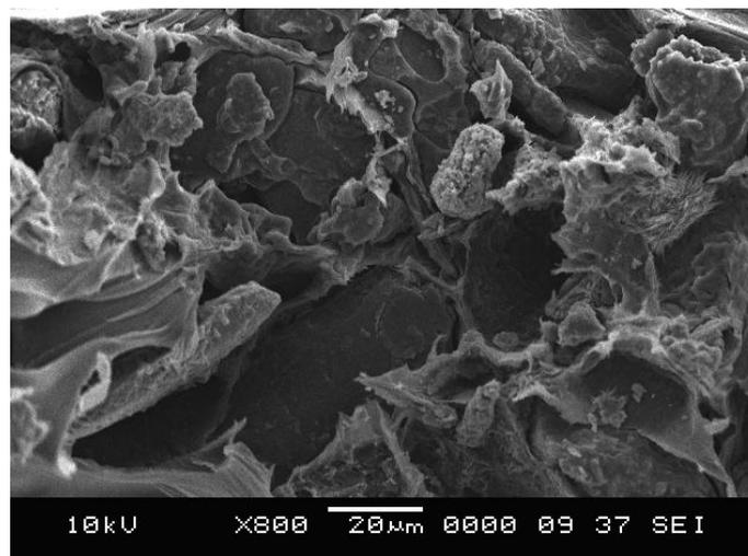
Fig. 4. SEM micrograph of untreated PLA/PKS biocomposite film (10 php PKS)
