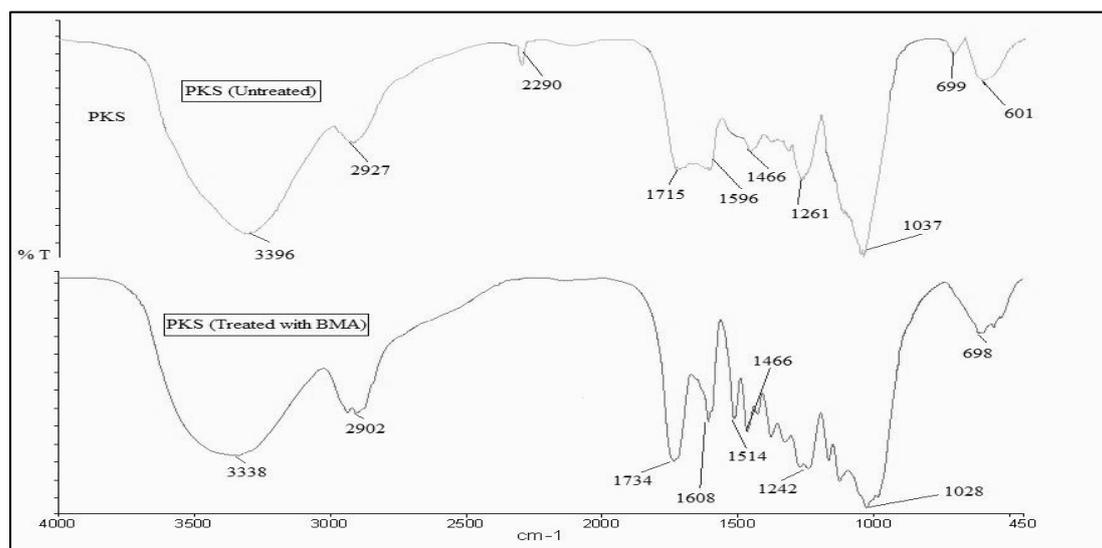
Fig. 6. FTIR spectra of untreated and treated PLA/PKS biocomposite films with BMA
