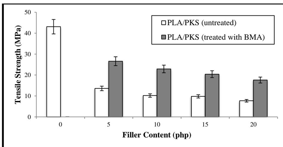
**Fig. 1.** Effect of filler content on the tensile strength of untreated and treated PLA/PKS biocomposite films
