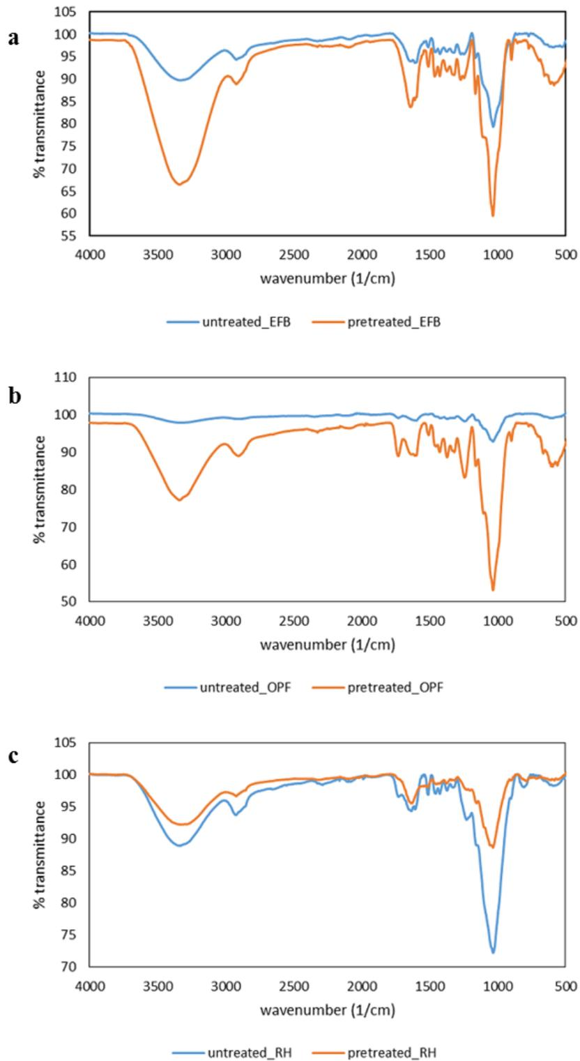
**Fig. 4.** FTIR spectra of alkali-pretreated SS samples: (a) EFB, (b) OPF, and (c) RH
