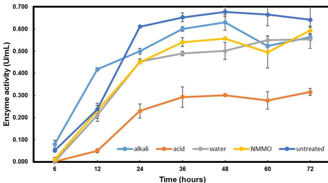
Fig. 2. Endoglucanase production by *B. aerius* S5.2 on pretreated and untreated MS samples
