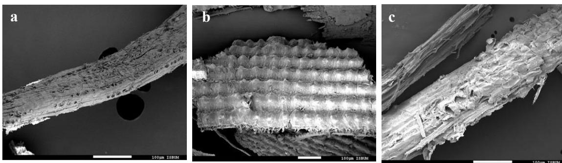
**Fig. 3.** FESEM micrographs of alkali-pretreated SS samples: (a) EFB x 250; (b) RH x 150; (c) OPF x 250
