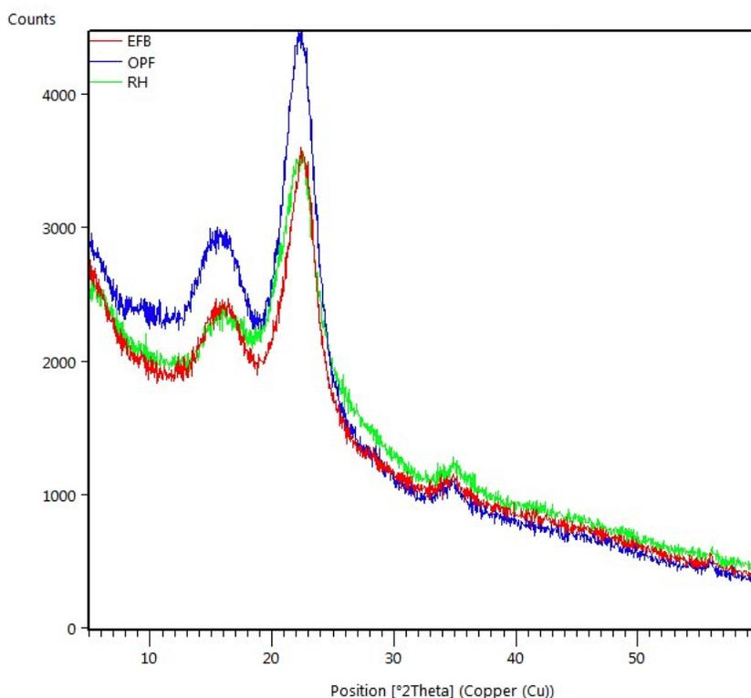
**Fig. 5.** XRD diffraction patterns of alkali-pretreated EFB, OPF, and RH
