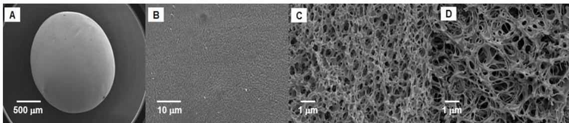
**Fig. 4.** Scanning electron microscope images of the modified xylan-PVOH beads. (A) morphology of the beads; (B) external surface at 2,000x magnification; (C) internal cross-section of the beads at 10,000x magnification; and (D) internal cross-section of PVOH beads at 5,500x magnification
