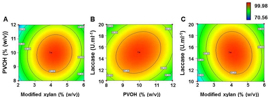
**Fig. 3.** Contour plots showing interactions between different concentrations of PVOH/xylan (A), laccase/PVOH (B), and laccase/xylan (C) on the response of RB-5 decolorization
