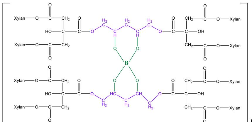
**Fig. 2.** Diagram of the modified xylan-PVOH bead structure. Modified xylan, PVOH, and boric acid are represented by the black, purple, and green sections, respectively.
