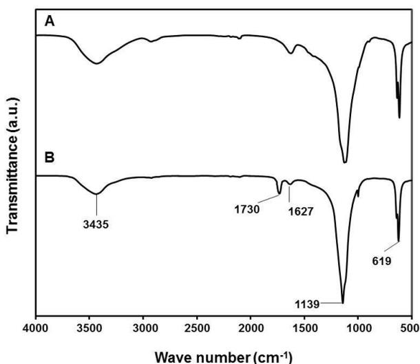
**Fig. 1.** FTIR spectra of the xylan isolated from black liquor of kraft pulping process of *Eucalyptus grandis* (A), and the modified xylan obtained from the esterification reaction with citric acid at 120 °C for 5 h (B)
