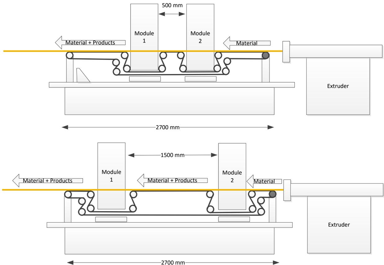
**Fig. 7.** Principle of 2-phase Kompoline process operation with an extruder and the proposed conveyor system. Press modules 1 and 2 move back and forth in relation to each other, while the composite web, marked in yellow, provides constant input from the extruder. The belt conveyor system consists of 13 idler pulleys and a drive pulley, illustrated in dark gray. The maximum distance between the press units in phase 1 and 2 is set to 1500 mm.
