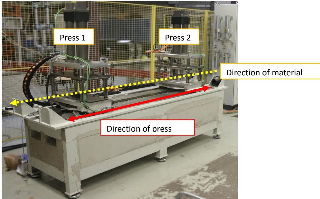
Fig. 5. LUT KompoLine press line with different elements illustrated
