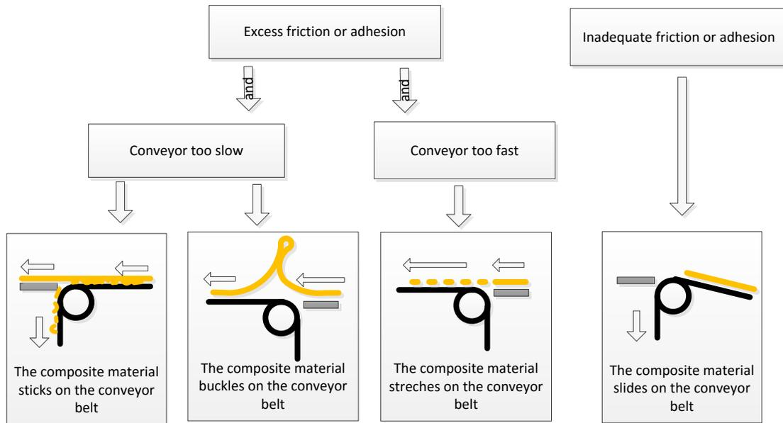
**Fig. 2.** Possible faults in conveying WPCs with a belt conveyor
