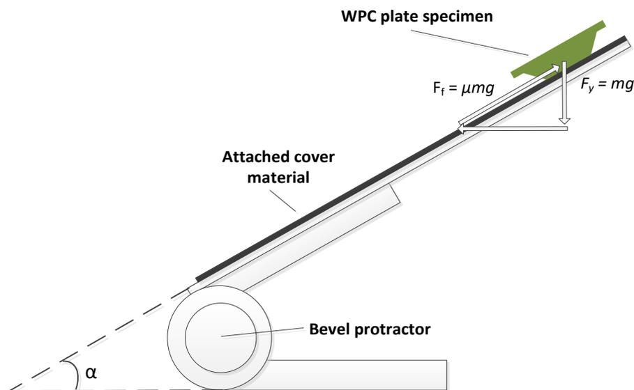
**Fig. 3.** Friction test setup based on an inclined plane and a bevel protractor based on TAPPI T815 (2006). The gravity force  $F_y$  causes the tested WPC material to slide at the angle where the friction force  $F_f$  is exceeded.
