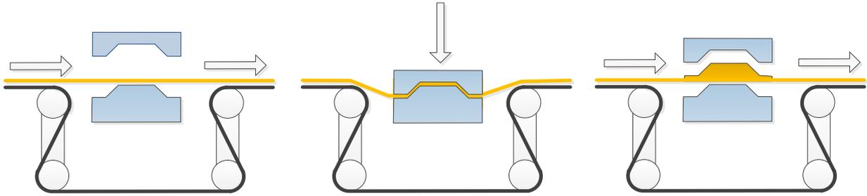
**Fig. 6.** A single pressing cycle for a WPC material web, illustrated in yellow, and press forming tools, in blue. The pressing event is illustrated in three stages relevant for the conveyor.
