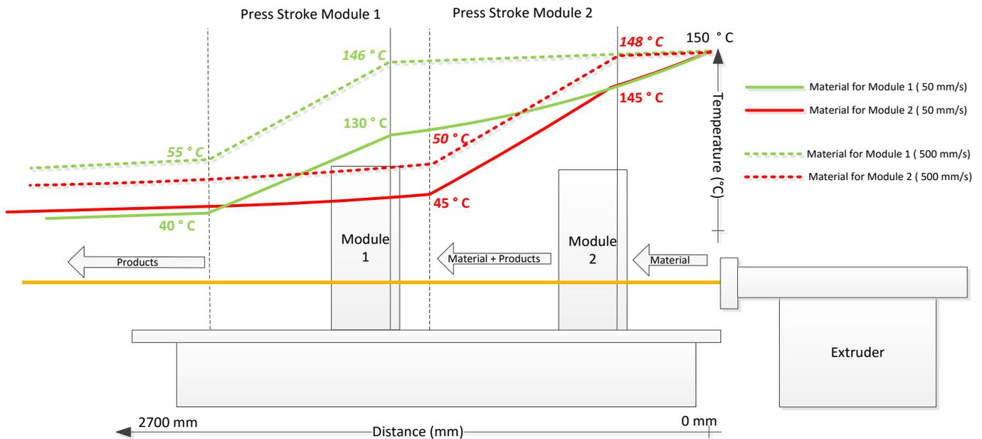
**Fig. 1.** Heat gradient across a post-extrusion process line used as a case example at two different extrusion speeds. The process line consists of two moving modules, described in experimental chapter under LUT KompoLine Platform- section. The yellow line illustrates the composite material web moving at the extrusion speed.
