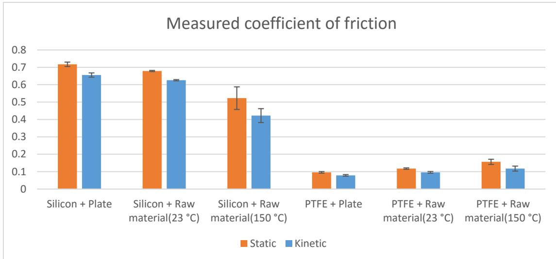
**Fig. 5.** Measured static and kinetic friction coefficients for the silicone and PTFE coated conveyor belts with standard deviation indicated.
