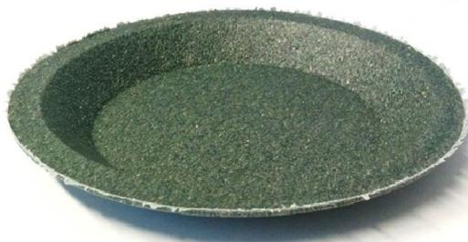
**Fig. 4.** Specimen plate made of thermoplastic WPC used in evaluation of friction and surface energy
