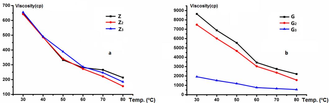
**Fig. 4.** Temperature dependence of 1.0% (w/v) solution viscosity for *G. microphylla* and guar gum solutions
