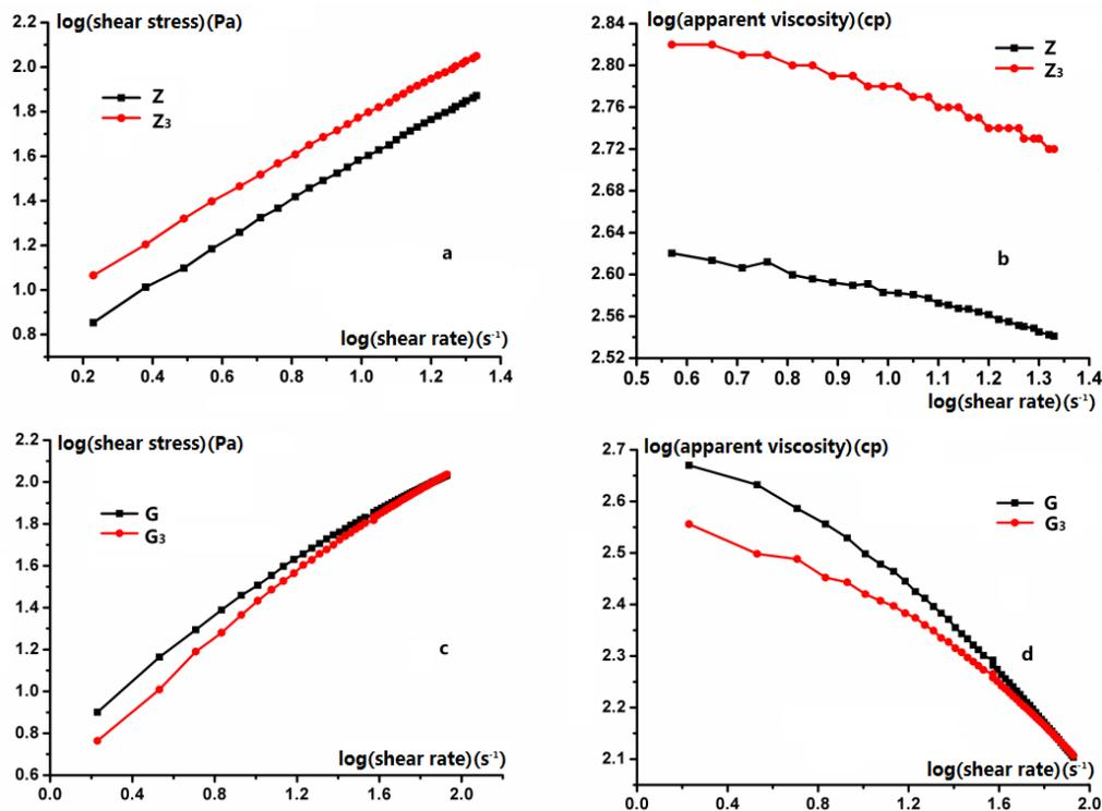
**Fig. 3.** Flow curves (a, c) and apparent viscosity curves (b, d) of 1% (w/v) *G. microphylla* gum (a, b) and guar gum (c, d) at 25 °C
