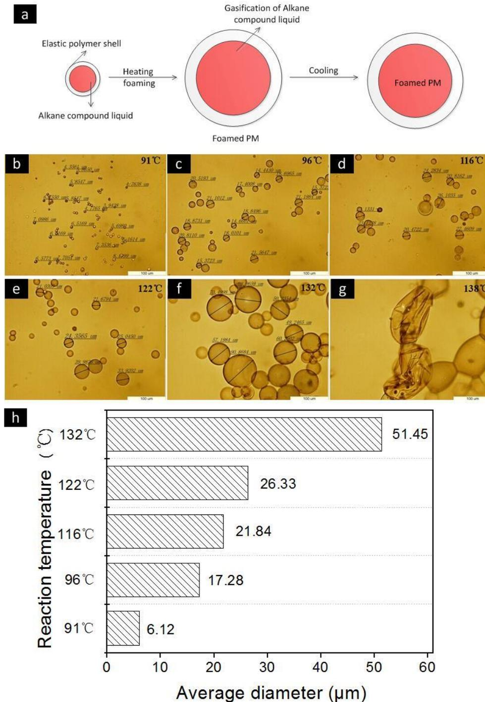
**Fig. 2.** (a) Schematic illustration of the foaming process of the PMs. The optical microscope pictures of PMs (e.g., F-36D model) were acquired at heating temperatures of (b) 91, (c) 96, (d) 116, (e) 122, (f) 132, and (g) 138 °C; (h) the average diameter of F-36D at different temperatures.
