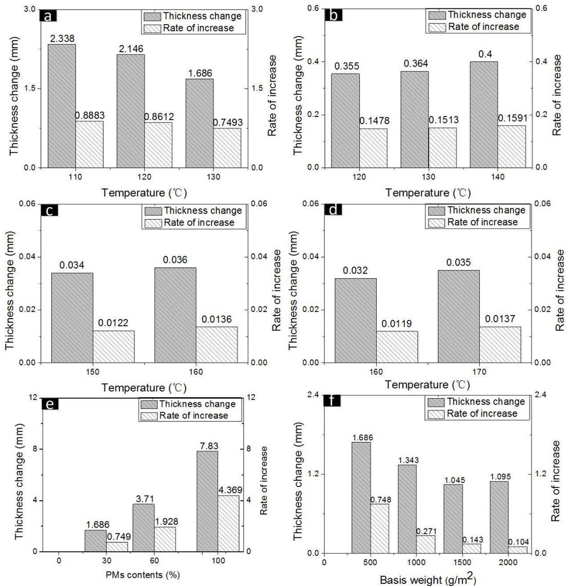
**Fig. 4.** Rate of increase and thickness change at (a) 110, 120, and 130 °C (F-36D), (b) 120, 130, and 140 °C (F-36), (c) 150 and 160 °C (F-48), and (d) 160 and 170 °C (F-50); (e) rate of increase and thickness change of F-36D with PM contents of 0, 30%, 60%, and 100%; (f) rate of increase and thickness change of F-36D with basis weights of 500, 1000, 1500, and 2000 g/m<sup>2</sup>
