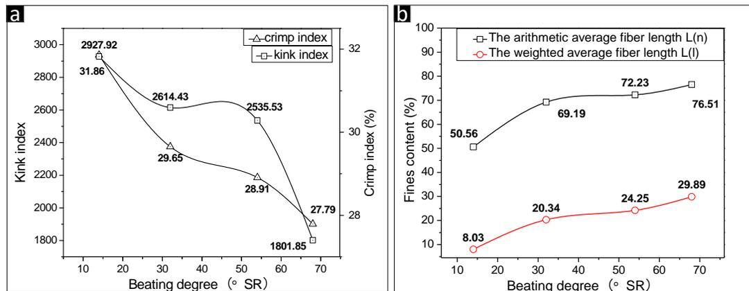
**Fig. 5.** (a) Kink index and crimp index at different beating degrees;(b) fines content at different beating degrees
