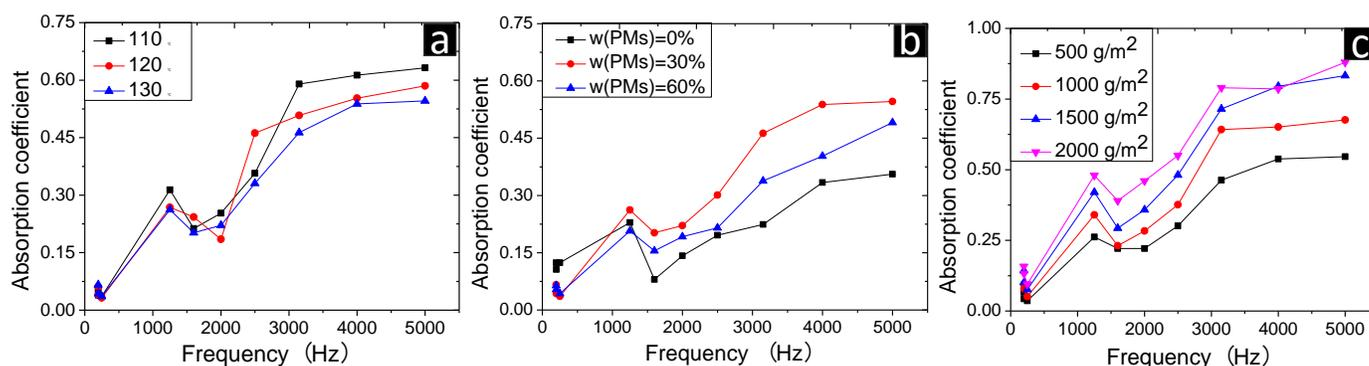
**Fig. 7.** Variation of the absorption coefficient with frequency at various (a) temperatures, (b) PM contents, and (c) basis weights.
