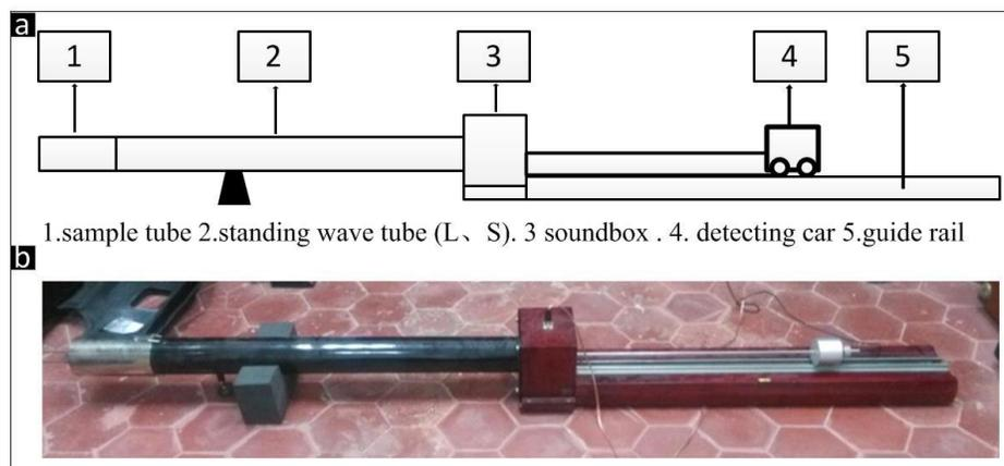
**Fig. 1.** (a) Schematic illustrating the working mechanism of acoustic tests. L standing wave tube is for low-frequency ( $\leq 1500$ Hz) test. S standing wave tube is for high-frequency ( $\geq 1500$  Hz) test; (b) picture of AWA6122 electroacoustic test system.
