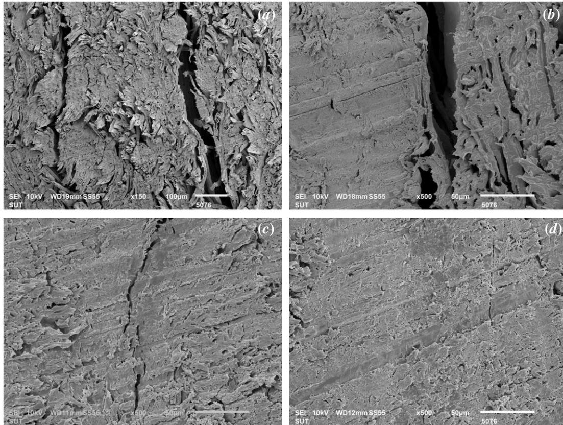
**Fig. 1.** SEM micrographs of eucalyptus wood foam (a) without OBSH at 150X, (b) without OBSH, at 500X, (c) with 3 phr OBSH, and (d) with 9 phr OBSH at 500X
