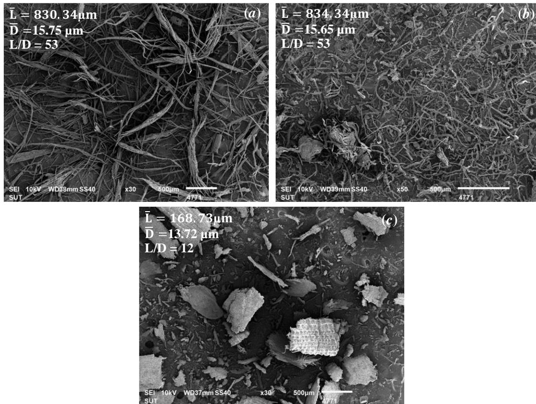
**Fig. 2.** SEM micrographs of (a) EF, (b) BG, and (c) RF
