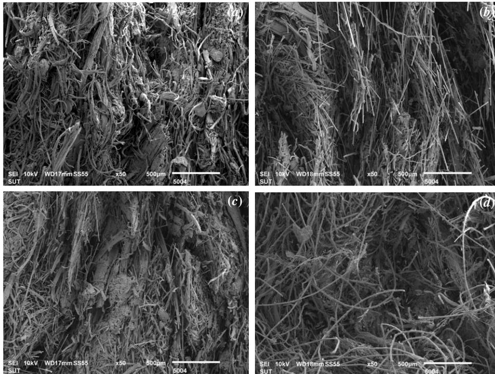
**Fig. 4.** SEM images of wood core made from (a) 50EF/50BG, (b) 35EF/35BG/30GF, (c) 35EF/35BG/30CF, and (d) 35EF/35BG/30KF at X50 $\times$
