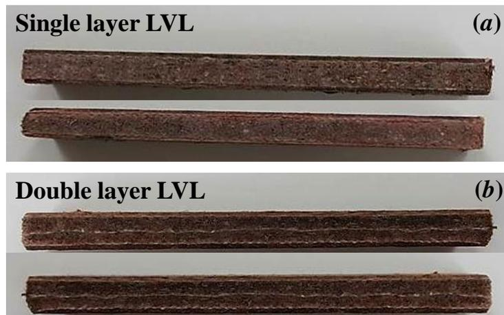
**Fig. 5.** Photographs of sandwich structure engineered wood reinforced with fiber glass products with; (a) single (1XLVL) and (b) double (2XLVL) layer core made from 50EF/50BG fibers
