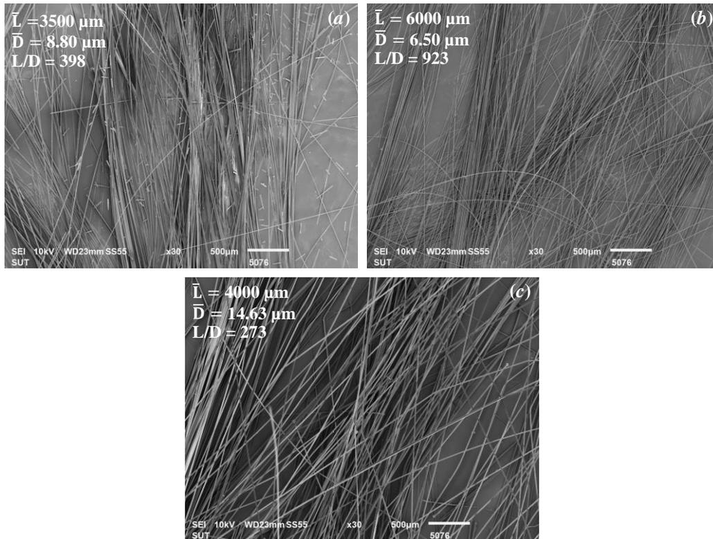
**Fig. 3.** SEM micrographs of (a) GF, (b) CF, and (c) KF fibers at 30 $\times$
