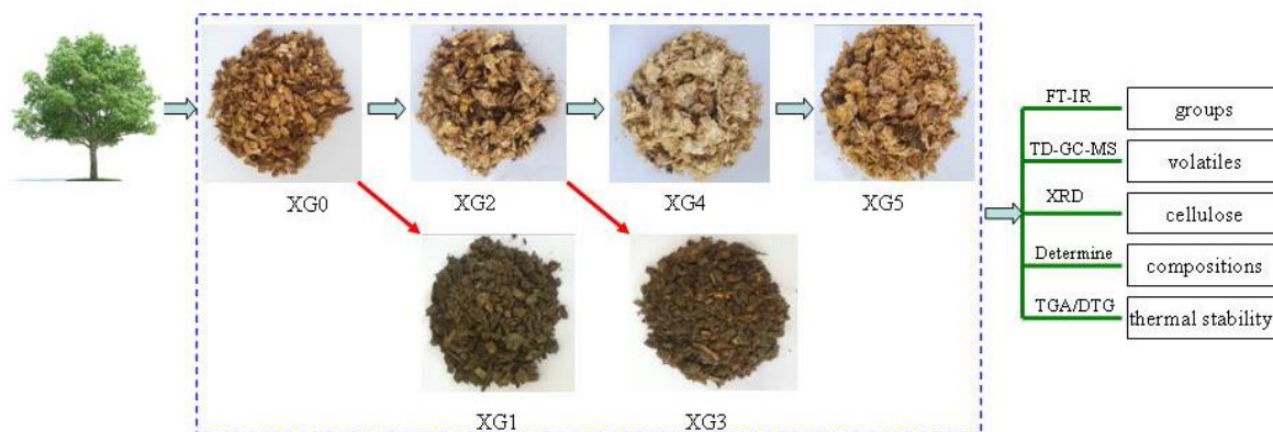
Fig. 1. Wood bioconversions during the artificial cultivation of L. edodes
