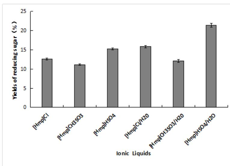
**Fig. 2.** Yields of reducing sugar in the pretreatment with IL. (0.25 g corn stalk, 5 g IL, 1 ml H<sub>2</sub>O, T=90 °C, t=30 min)
