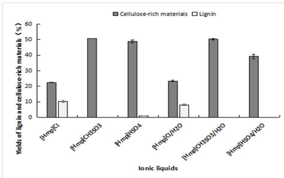
**Fig. 1.** Yields of lignin and cellulose-rich materials extracted from corn stalk with IL and IL/H<sub>2</sub>O. (0.25 g corn stalk, 5 g IL, 1 ml H<sub>2</sub>O, T=90 °C , t=30 min)
