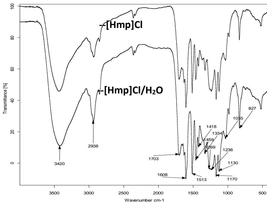
**Fig. 4.** FTIR spectra of lignin extracted from corn stalk with [Hmp]Cl and [Hmp]Cl/H<sub>2</sub>O. (0.25 g corn stalk, 5 g [Hmp]Cl, 1 mL H<sub>2</sub>O,  $T=90\text{ }^{\circ}\text{C}$ ,  $t=30\text{ min}$ )
