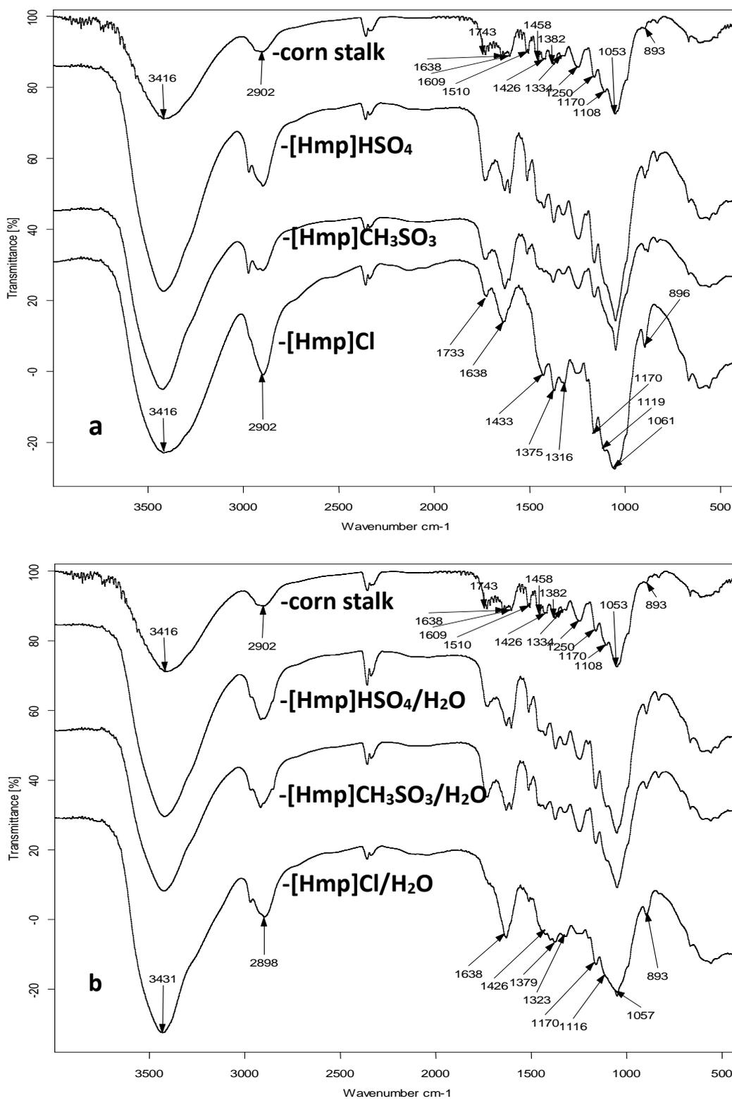
**Fig. 3.** FTIR spectra of untreated corn stalk and cellulose-rich materials extracted from corn stalk with IL (a) and IL/H<sub>2</sub>O (b). (0.25 g corn stalk, 5 g IL, 1 mL H<sub>2</sub>O,  $T=90$  °C,  $t=30$  min)
