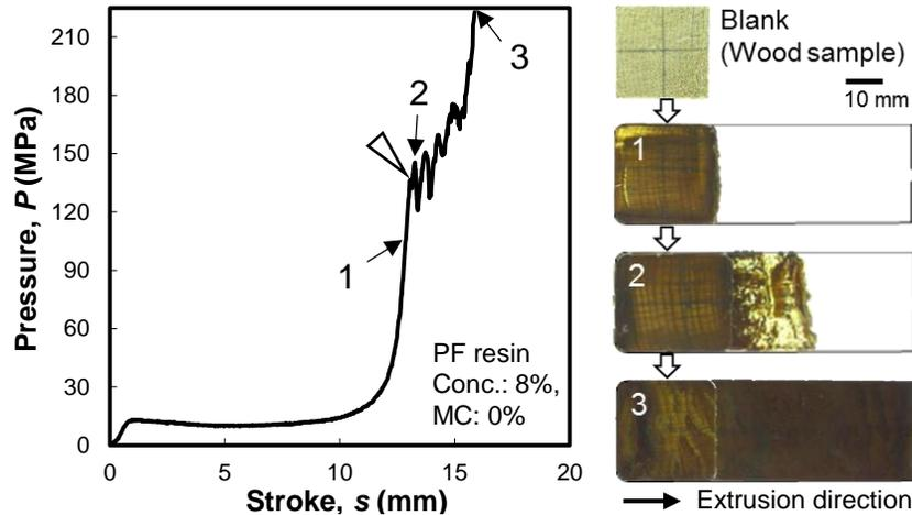
**Fig. 4.** Punch pressure and wood deformation behavior during the extrusion test (PF resin concentration: 8%, MC: 0%). A triangle denotes the starting point of extrusion.
