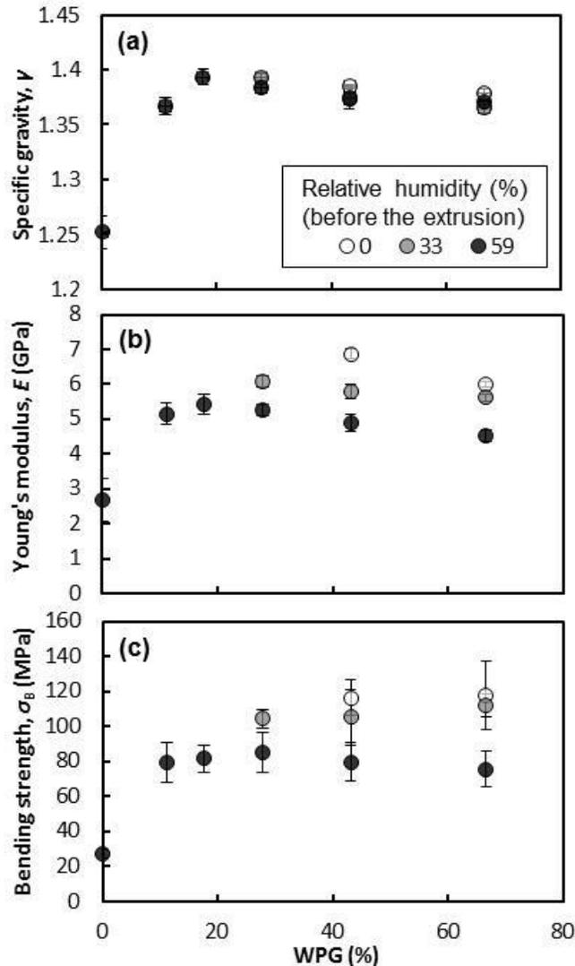
**Fig. 7.** Relationships between WPG of the wood samples due to PF resin impregnation and specific gravity ( $\gamma$ ), Young's modulus ( $E$ ), and bending strength ( $\sigma_B$ ) of the extrudate obtained from the wood samples conditioned at different relative humidities (RHs)
