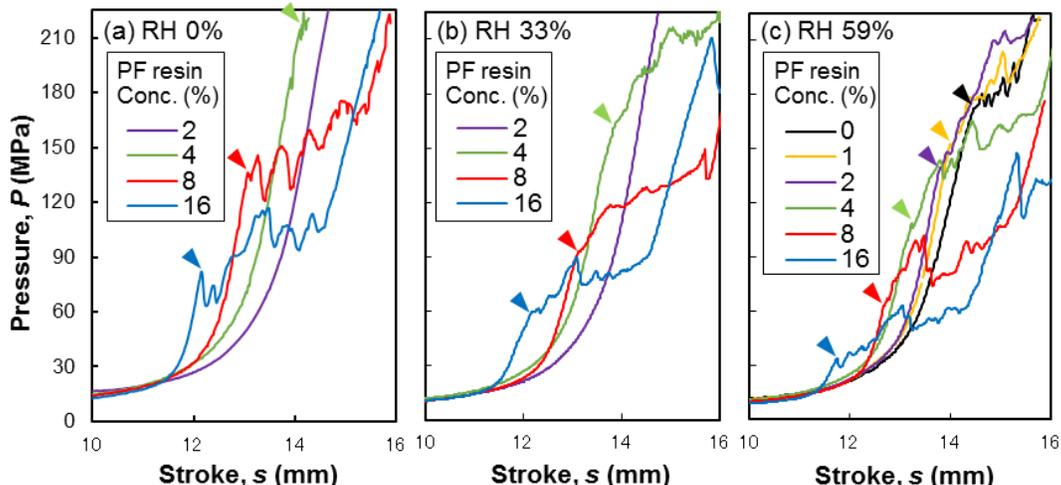
**Fig. 5.** Comparison of punch pressure behavior during the extrusion test of wood samples prepared with different PF resin concentrations and relative humidities (RHs). A triangle denotes the starting point of an extrusion.
