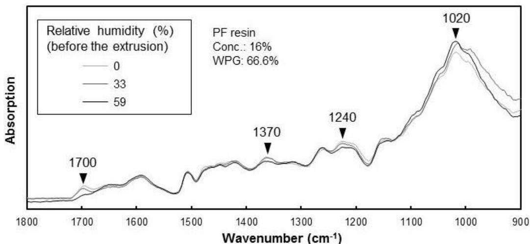
**Fig. 10.** FTIR spectra of extrudates obtained from wood samples conditioned at different relative humidities (RHs)
