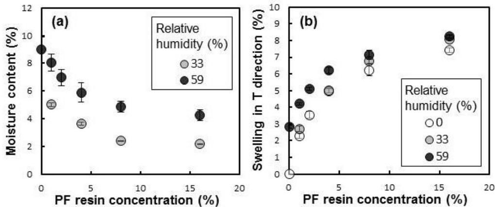
**Fig. 3.** Relationships between PF resin concentration and moisture content (a) and swelling in T direction (b) of the wood samples
