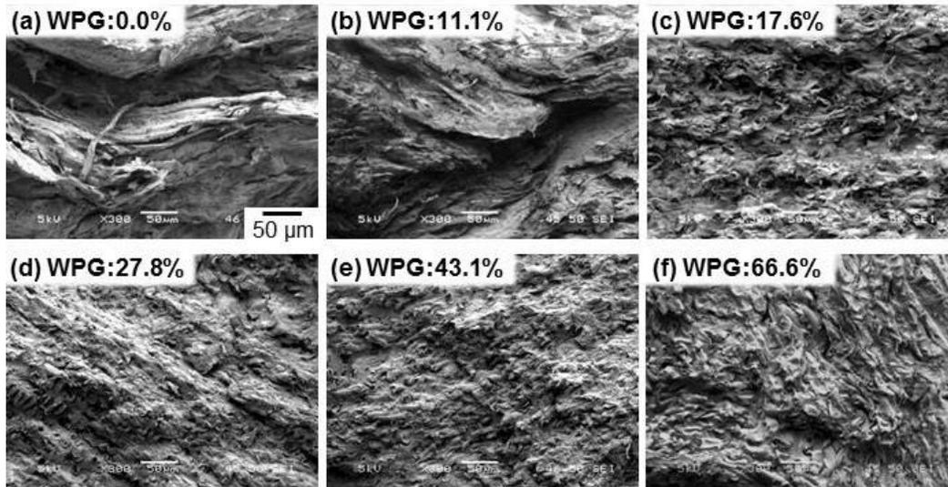
**Fig. 8.** SEM micrographs of fracture surface of extrudates obtained from wood samples conditioned at 59% RH
