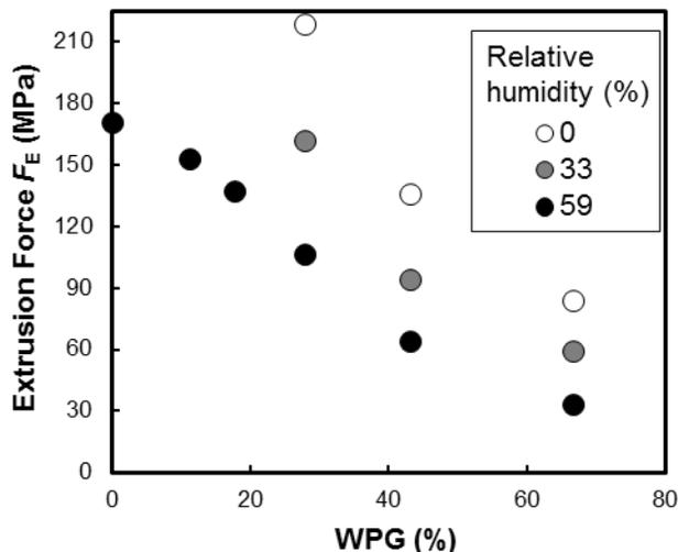
**Fig. 6.** Relationship between WPG of the wood samples due to PF resin impregnation and extrusion force ( $F_E$ ) of wood samples prepared with various relative humidities (RHs)
