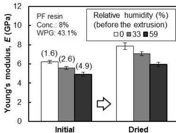
**Fig. 9.** Changes of Young's modulus of the extrudates before (Initial) and after drying (Dried) treatments. The extrudates were obtained from the wood samples impregnated with a PF resin concentration of 8% and conditioned at different relative humidities (RHs). The values given in parentheses are the residual moisture contents (RMCs) of the extrudates at the initial state.
