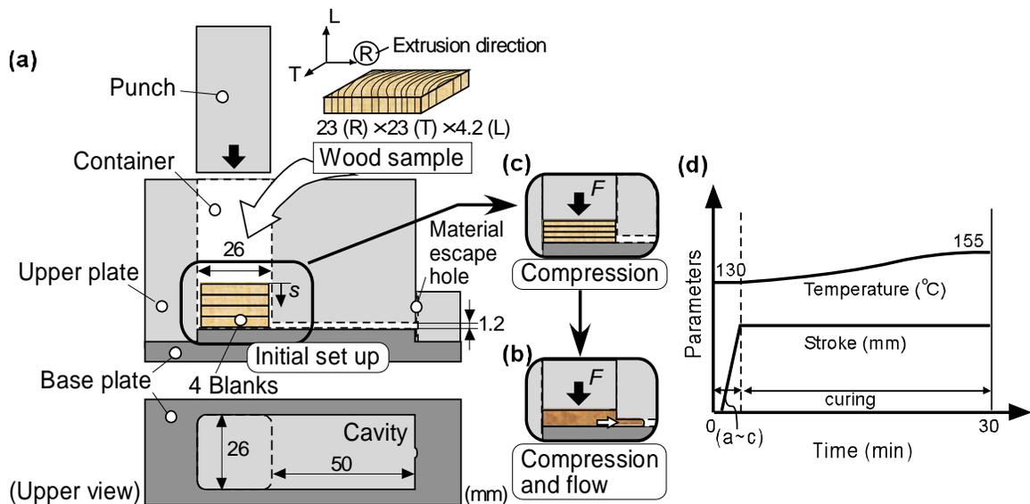
**Fig. 1.** Schematic illustration of the extrusion process. (a to c) Metal mold used for the extrusion test. (d) Wood deformation behavior and parameter changes during the extrusion process
