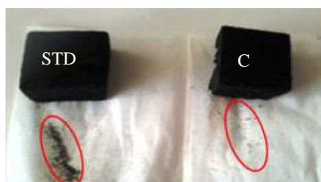
Fig. 6. Friability of standard foam (STD) and foam C
