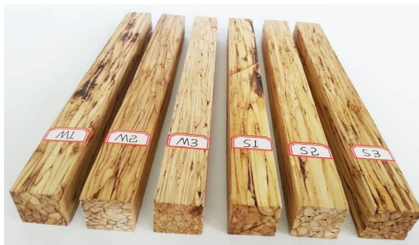
Fig. 4. Bending test specimens of lumber made from cotton stalks and mulberry branches
