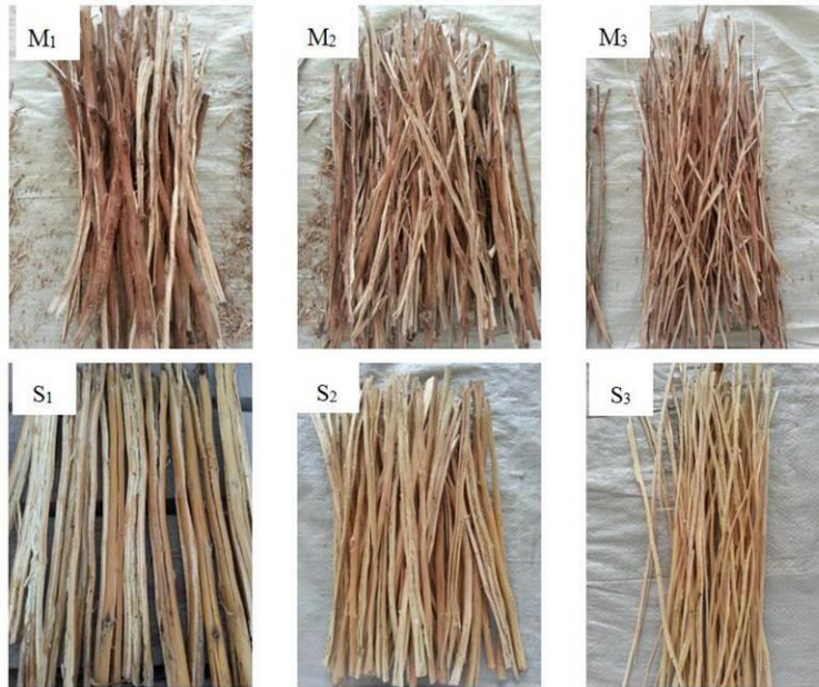
Fig. 2. Cotton stalk and mulberry branch fiber bundles with different L/T ratios. Thick cotton stalk ( M_1 ), medium cotton stalk ( M_2 ), thin cotton stalk ( M_3 ), thick mulberry branch ( S_1 ), medium mulberry branch ( S_2 ), and thin mulberry branch ( S_3 )
