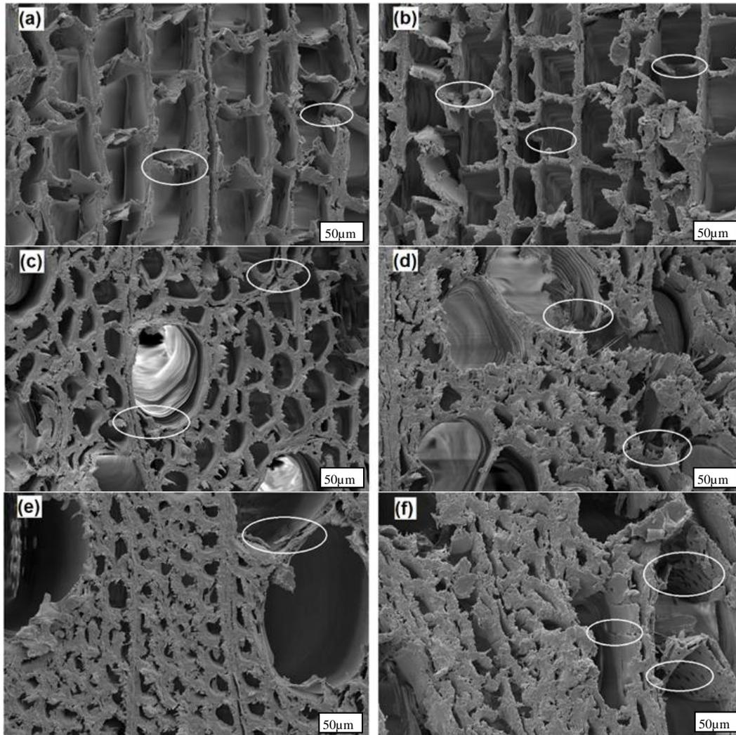
**Fig. 6.** Scanning electron microscope images in cross-sections of samples subjected only to heat treatment: a) Uludağ fir heat-treated at 185 °C; b) Uludağ fir heat-treated at 212 °C; c) linden heat-treated at 185 °C; d) linden heat-treated at 212 °C; e) black poplar heat-treated at 185 °C; f) black poplar heat-treated at 212 °C
