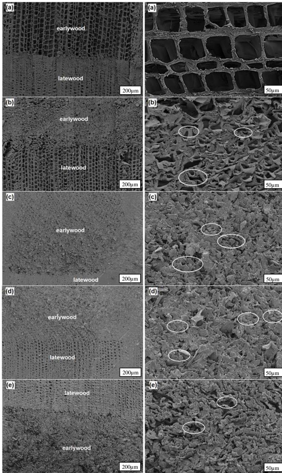
**Fig. 5.** Scanning electron microscope images of cross-sections of Uludağ fir wood samples: a) control (untreated); b) 25% compressed at 100 °C; c) 50% compressed at 100 °C; d) 50% compressed at 140 °C; e) 50% compressed at 140 °C and heat post-treated at 212 °C
