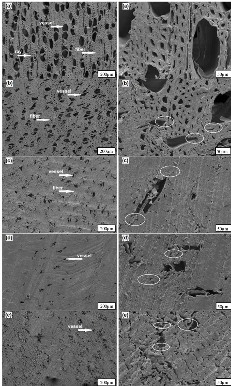
**Fig. 4.** Scanning electron microscope images of cross-sections of black poplar wood samples: a) control (untreated); b) 25% compressed at 100 °C; c) 50% compressed at 100 °C; d) 50% compressed at 140 °C; e) 50% compressed at 140 °C and heat post-treated at 212 °C
