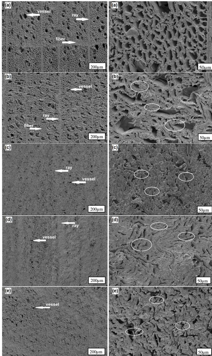
**Fig. 3.** Scanning electron microscope images of cross-sections of linden wood samples: a) control (untreated); b) 25% compressed at 100 °C; c) 50% compressed at 100 °C; d) 50% compressed at 140 °C; e) 50% compressed at 140 °C and heat post-treated at 212 °C
