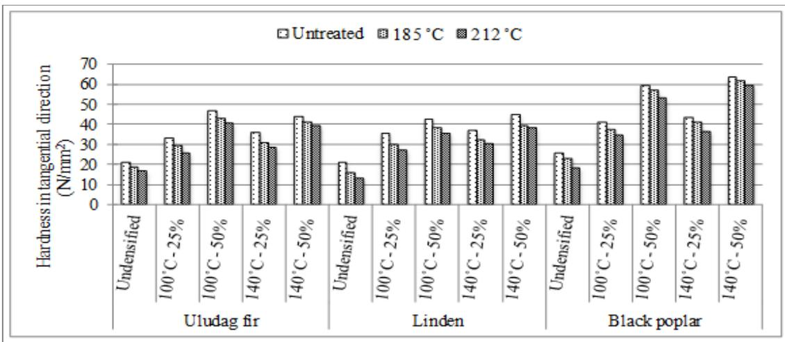
Fig. 2. Comparison of the hardness measurements in the tangential direction
