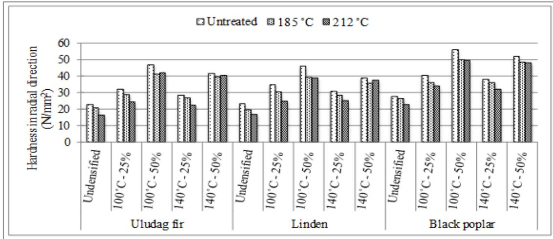
Fig. 1. Comparison of the hardness measurements in the radial direction
