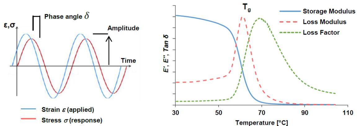
Fig. 1. a) DMA signals; b) typical storage modulus, loss modulus, and loss factor of EPX
