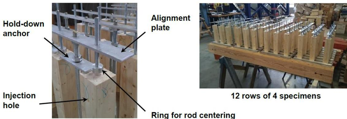
Fig. 4. Setup for fabrication of glued-in rod specimens
