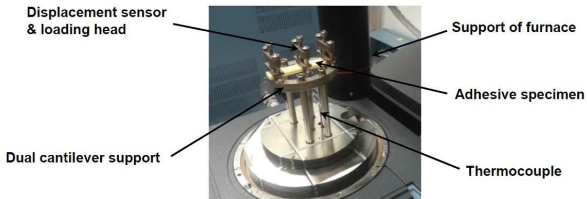
Fig. 2. Dual cantilever support with a specimen in the Q800 DMA testing machine
