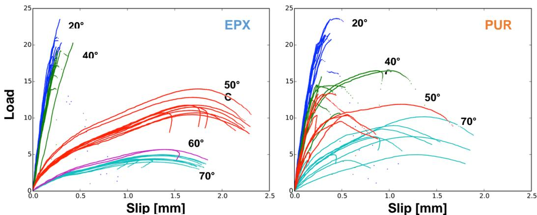
Fig. 9. Load/slip curves of glued-in rod connections tested at different temperatures
