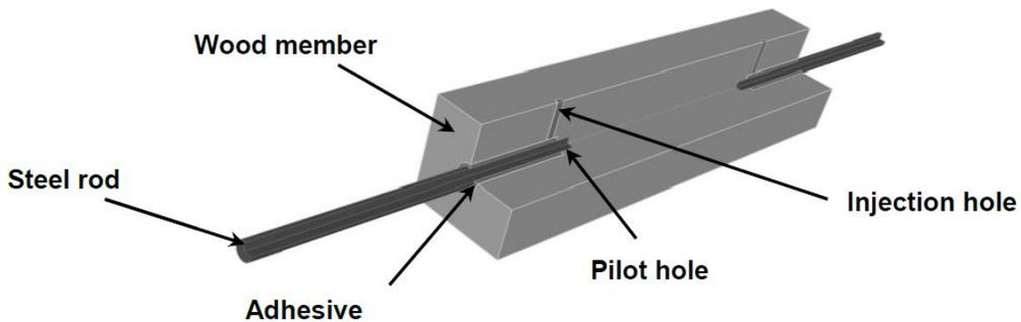
Fig. 3. Specimen of glued-in rod connection (pull-pull configuration)
