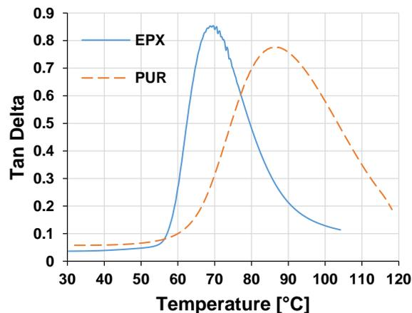
Fig. 6. Evolution of the loss factor with the increasing temperature for PUR and EPX
