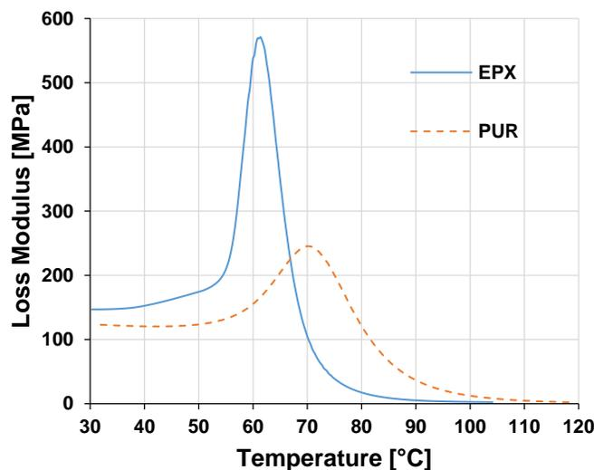
Fig. 8. Evolution of the loss modulus with the increasing temperature for EPX and PUR
