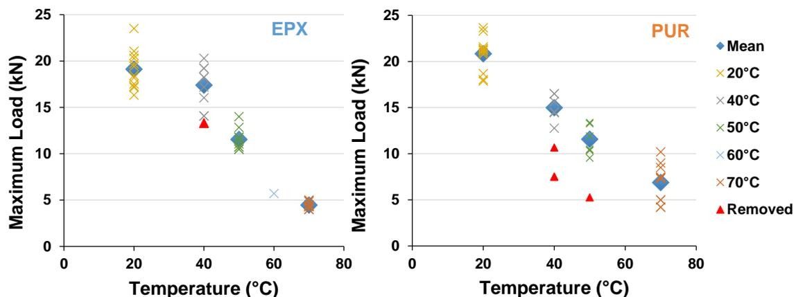
**Fig. 11.** Maximum loads of EPX and PUR glued-in rod connections tested at different temperatures
