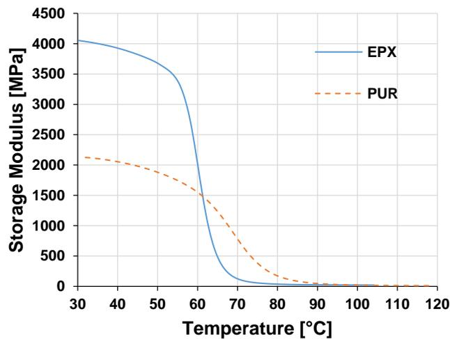
Fig. 7. Evolution of the storage modulus with the increasing temperature for EPX and PUR
