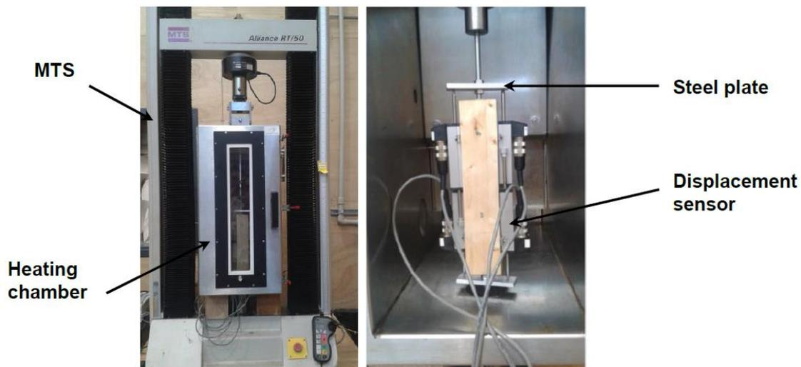
**Fig. 5.** a) Set up on MTS press; b) instrumented glued-in rod specimen
