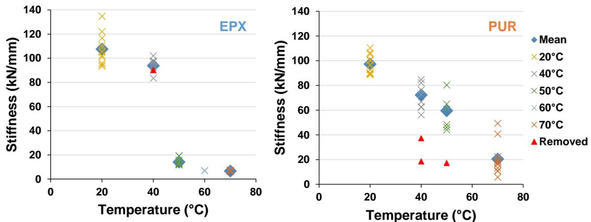
Fig. 10. Stiffness of EPX and PUR glued-in rod connections tested at different temperatures
