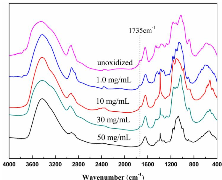
Fig. 2. FT-IR spectra of the unoxidized and oxidized bamboo pulp fibers
