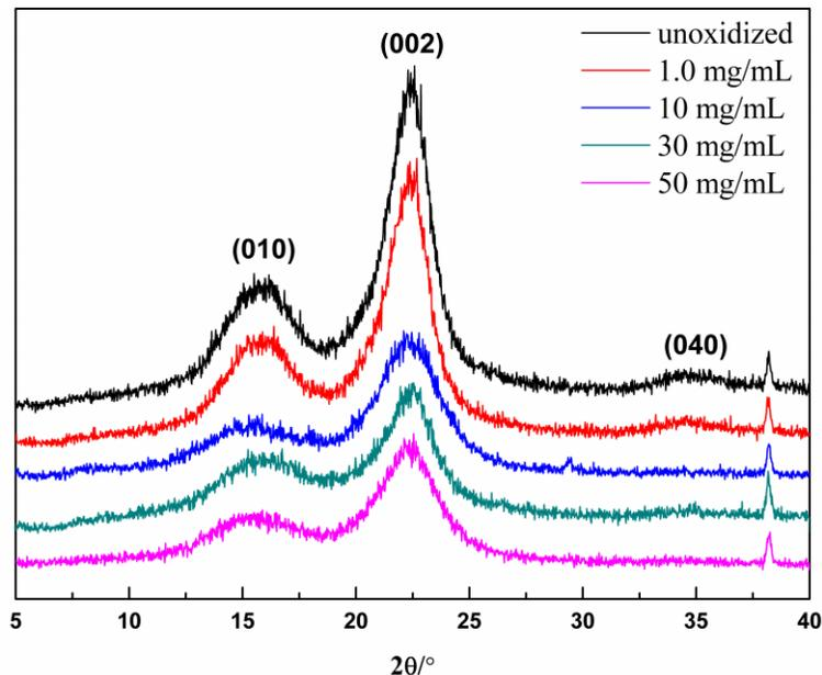
Fig. 3. XRD patterns of bamboo fibers with and without  $\text{NaIO}_4$  oxidation
