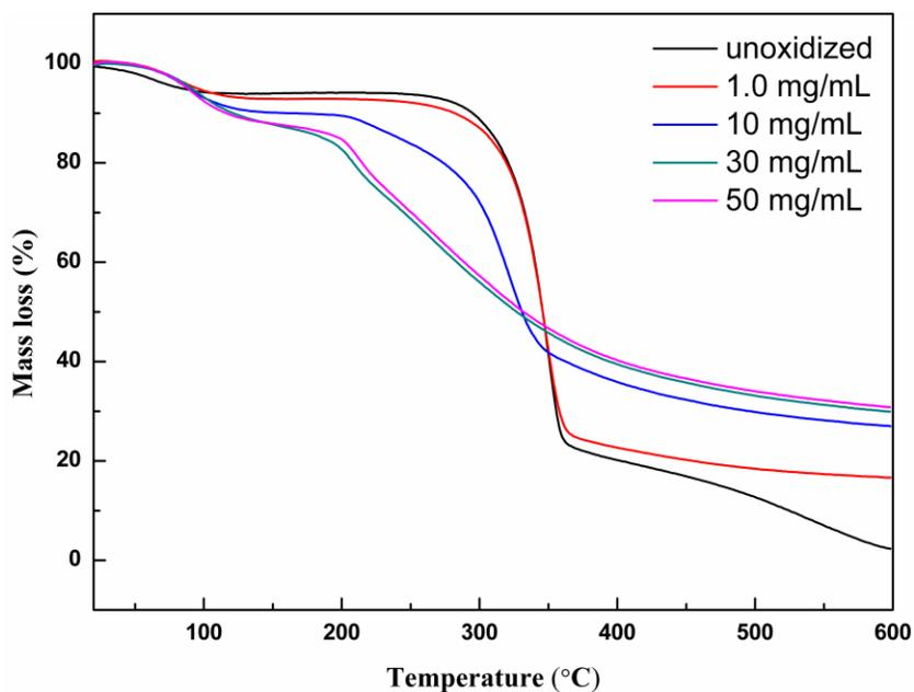
Fig. 5. TGA curves of bamboo fibers with and without  $\text{NaIO}_4$  oxidization
