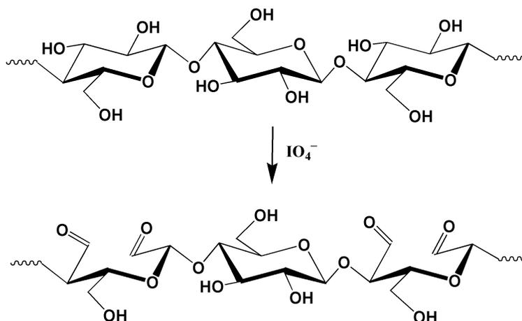
Fig. 1. Schematic of preparation of cellulose oxidized by periodates
