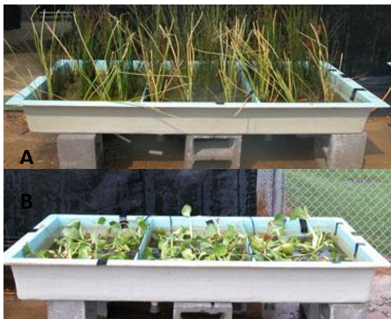
Fig. 3. Emergent (A) and Floating (B) wetlands were established in fiberglass tubs divided into three sections. Each section was filled with OSB process wastewater plus plants and served as a replicate.
