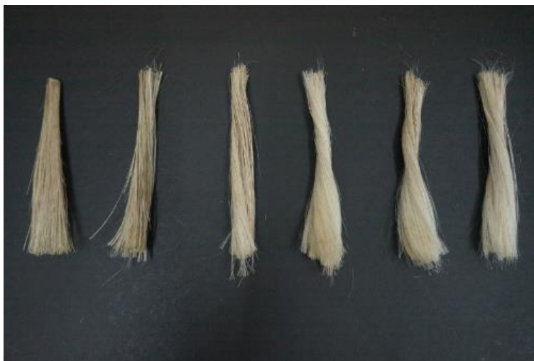
Fig. 1. Pectinase-treated kenaf fibres; from left to right: untreated, 8 h, 16 h, 24 h, 32 h, and 40 h treatment with A. fumigatus R6 pectinase
