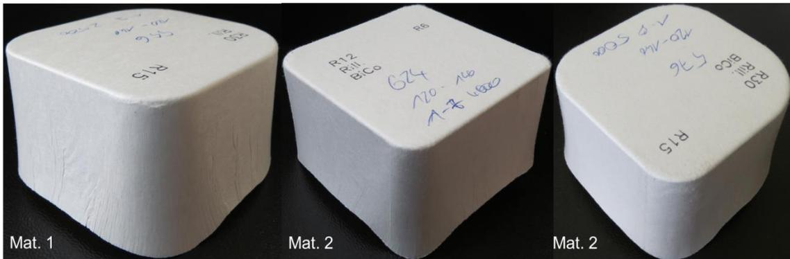
**Fig. 12.** Samples of rectangular 3D-shapes made with the toolsets introduced in Fig. 1 from material 1 (left) with 15 mm radius in front and from material 2 (middle with radius 10 mm in front and right with radius 15 mm in front)
