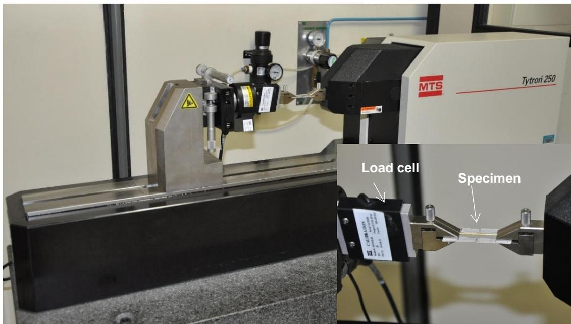
**Fig. 2.** The direct tensile test setup of the MTS Tytron 250 and a zoom in showing the load cell and the peach palm fiber specimen
