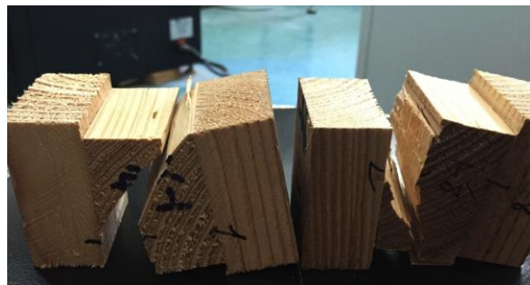
Fig. 3. The failure model of block shear strength for CLT
