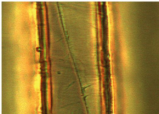
**Fig. 2.** Tangential cross-section of a spruce wood sample subjected to  $\text{CoCl}_2$ , showing a crack along the microfibrils
