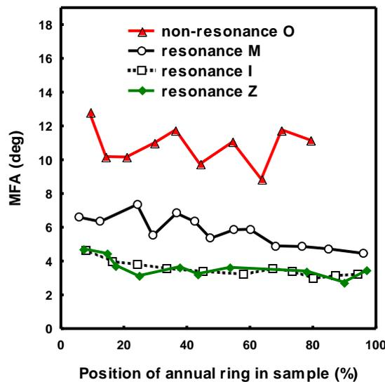
Fig. 5. Average MFA in the annual rings versus the position of the ring in the sample: M - Mazoče; I - Istebna; Z - Zvolen; O – Olsztyn
