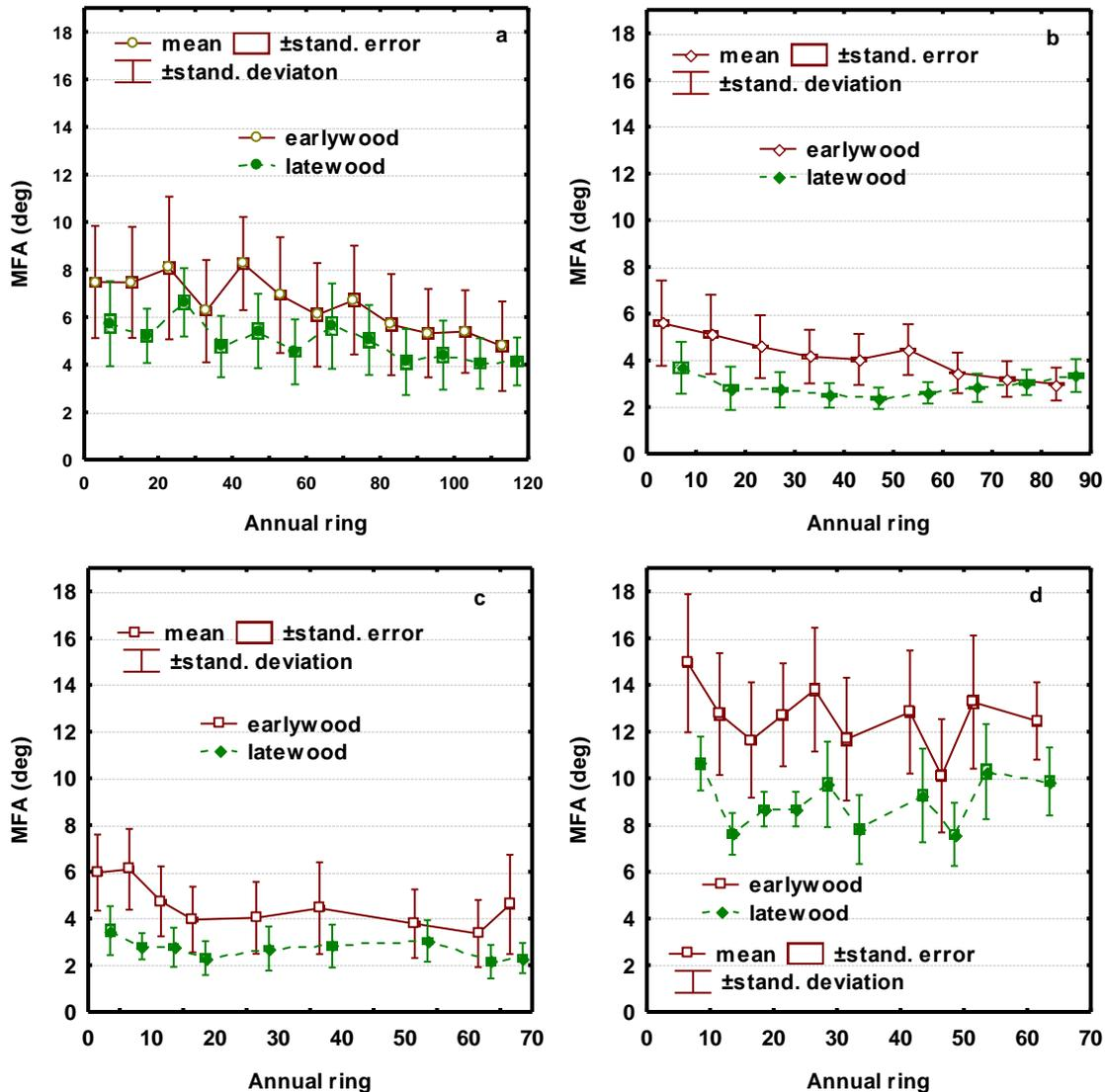
**Fig. 3.** Mean MFA in early- and latewood tracheids in the resonance samples from a) Mazoče, b) Istebna, c) Zvolen, and non-resonance samples d) from Olsztyn. (The OX axis gives subsequent number of annual ring in a given sample)
