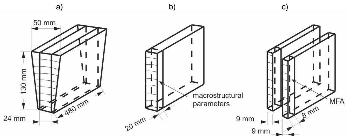
Fig. 1. Diagram of sample cutting
