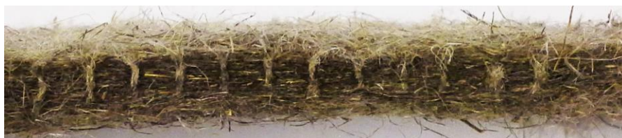
Fig. 3. Section of a reinforced mat
