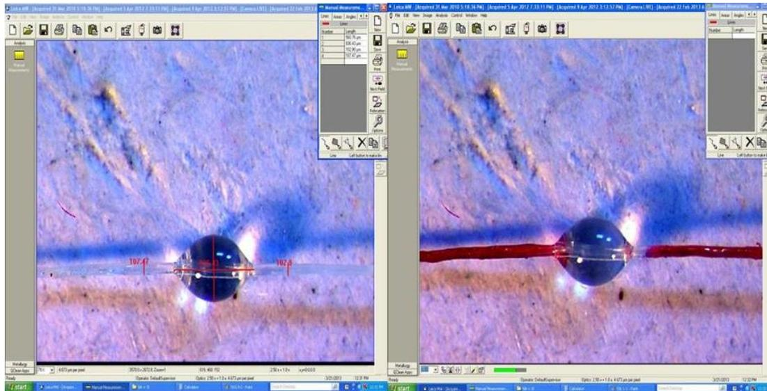
**Fig. 4.** Micro-droplet specimen
