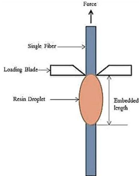
**Fig. 3.** Schematic of the micro-droplet test
