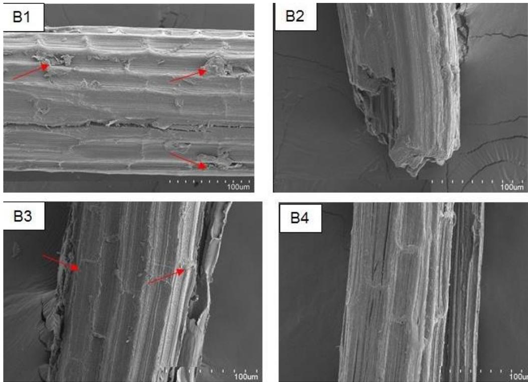
**Fig. 8B.** STOX (B1) Untreated sisal, (B2) sisal treated with NaOH, (B3) sisal treated with silane, and (B4) sisal treated with NaOH followed by silane. Arrows denote impurities on the samples
