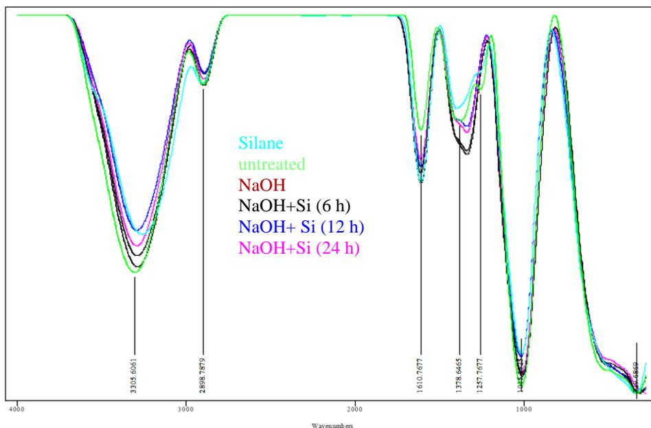
Fig. 7. FTIR spectra for untreated and treated fibers
