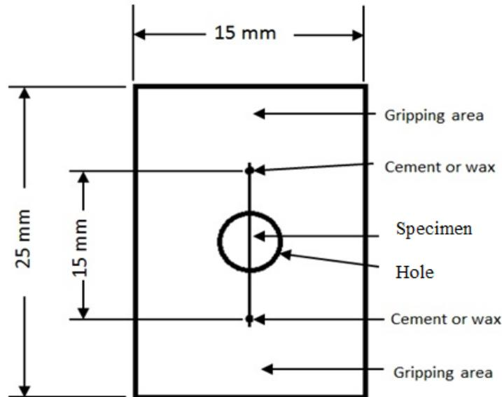
**Fig. 2.** Schematic of single-fibre tensile test sample
