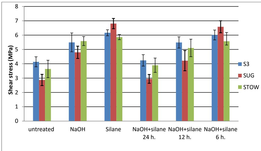
Fig. 6. Interfacial shear strength. Data provided as the mean  $\pm$  standard deviation
