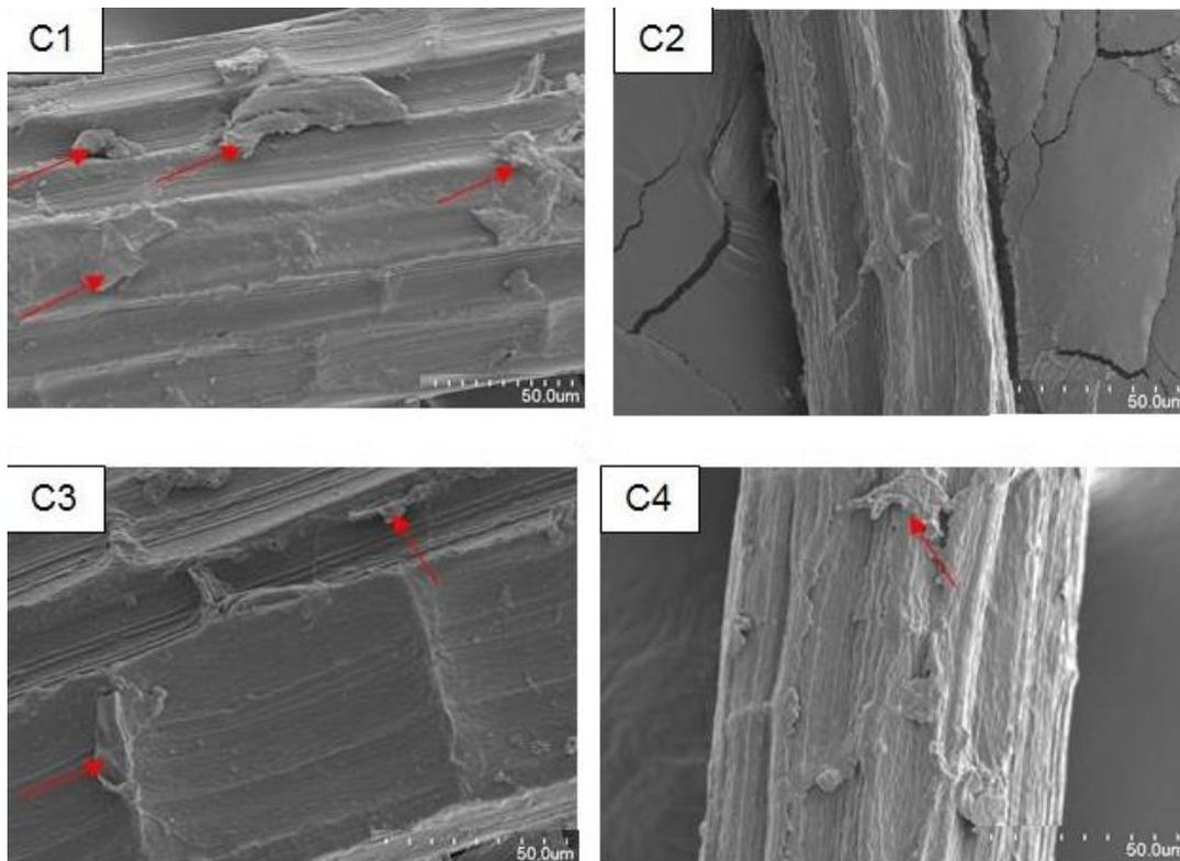
**Fig. 8C.** SUG (C1) Untreated sisal, (C2) sisal treated with NaOH, (C3) sisal treated with silane, and (C4) sisal treated with NaOH followed by silane. Arrows denote impurities on the samples.
