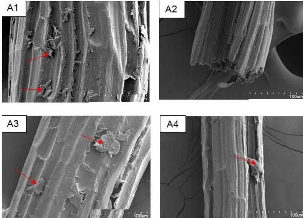
**Fig. 8A.** SEM images S3. (A1) Untreated sisal, (A2) sisal treated with NaOH, (A3) sisal treated with silane, and (A4) sisal treated with NaOH followed by silane. Arrows denote impurities on the samples
