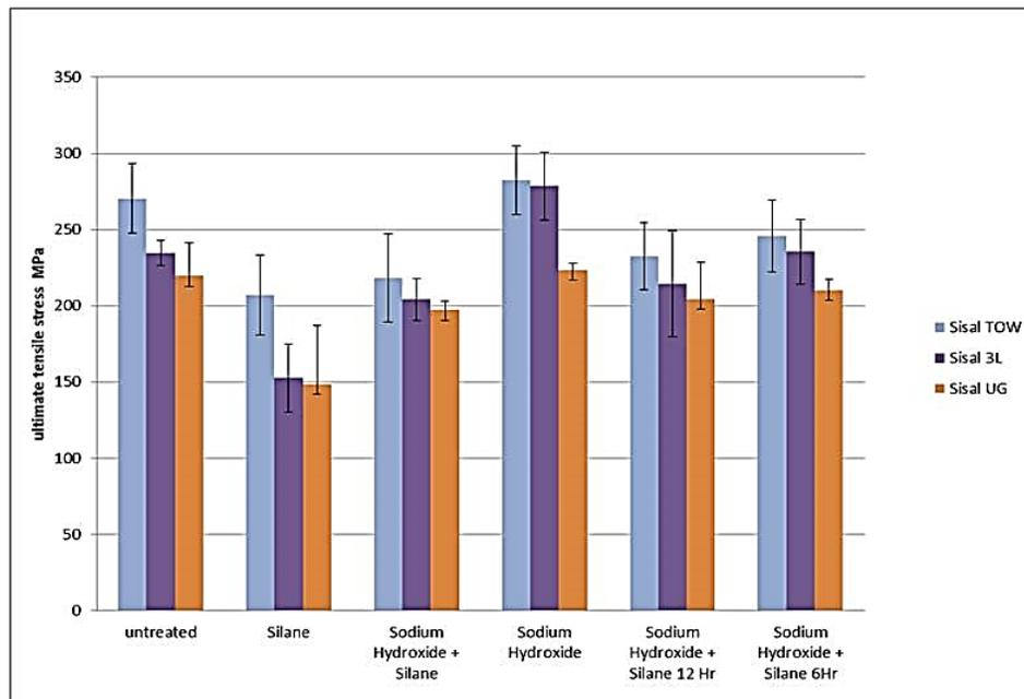
**Fig. 5.** Ultimate tensile stress. Data provided as the mean  $\pm$  standard deviation
