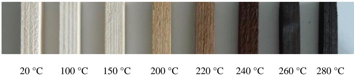
Fig. 1. Influence of treatment temperature on the color of fir wood
