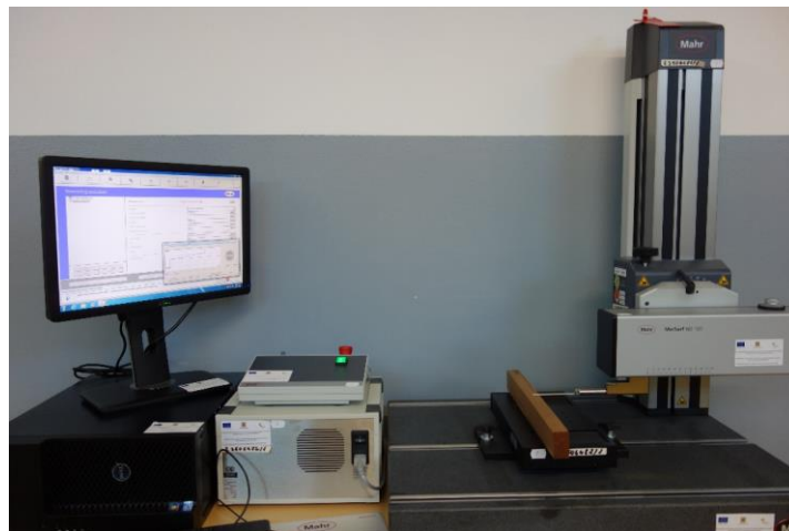
Fig. 3. MarSurf XT20 instrument used to measure the roughness parameters of the processed surface
