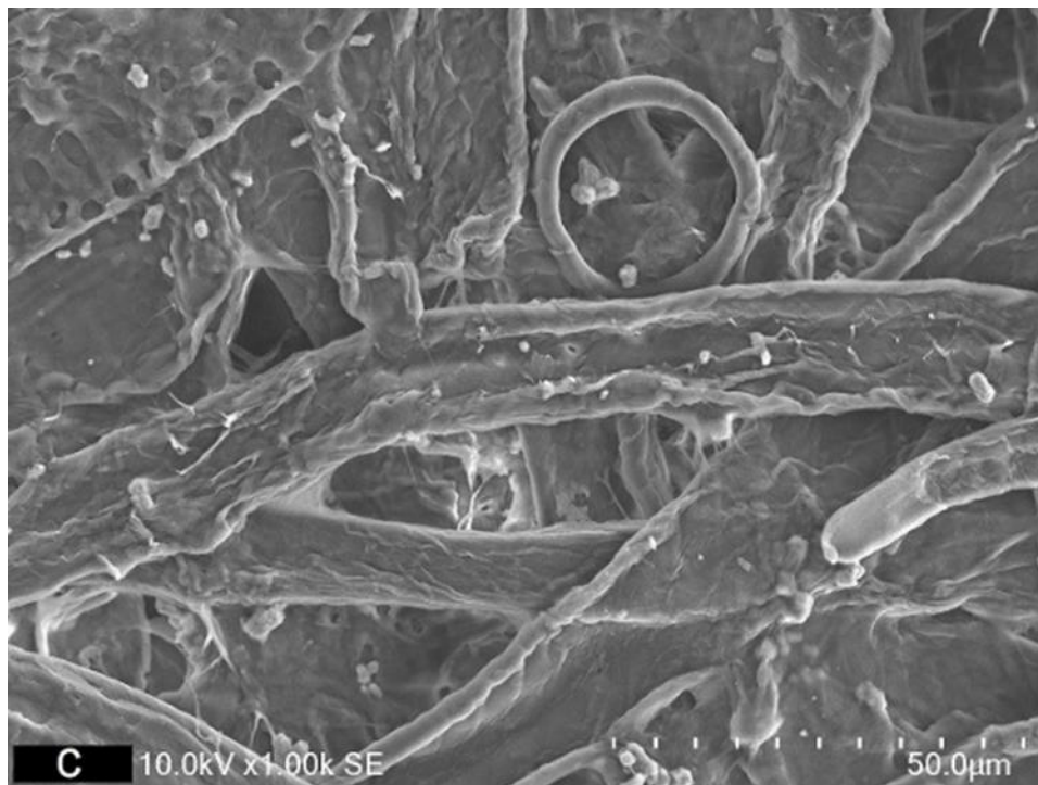
Fig. 2(c). Scanning electron micrographs of the bagasse paper (a, b) and bagasse paper with cellulose nanofibers and cationic polyacrylamide (c, d)
