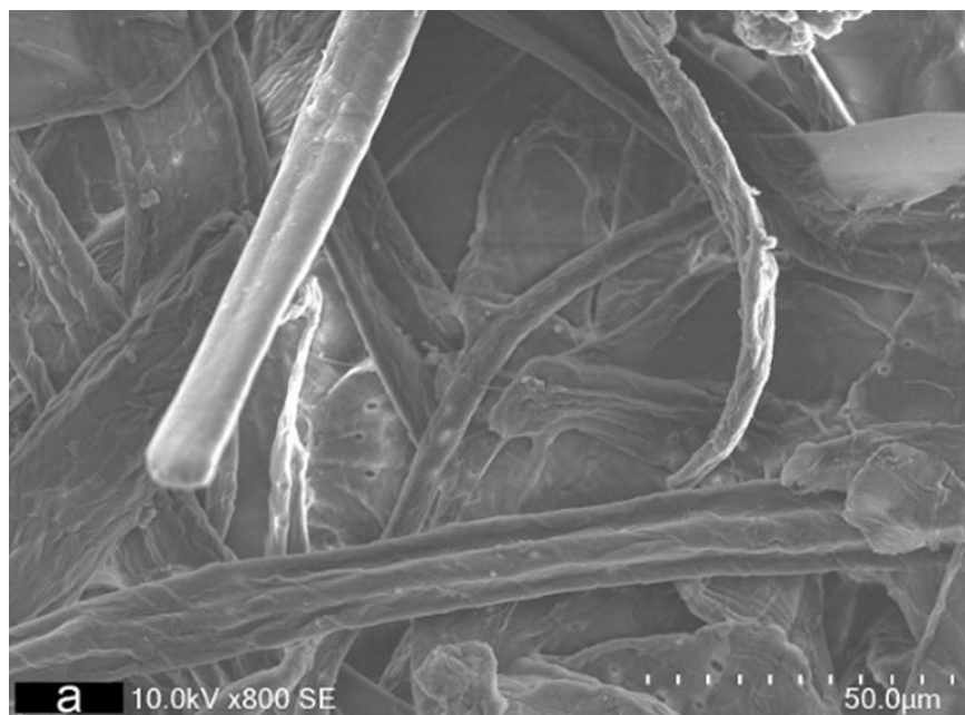
Fig. 2(a). Scanning electron micrographs of the bagasse paper (a, b) and bagasse paper with cellulose nanofibers and cationic polyacrylamide (c, d)
