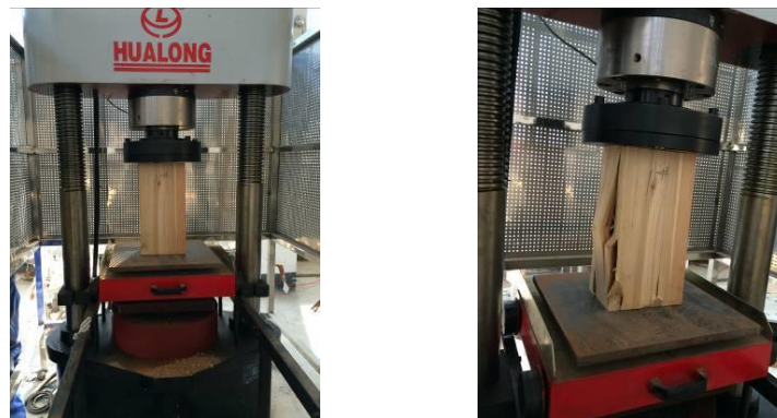
Fig. 2. Compressive strength full scale tests of timber
