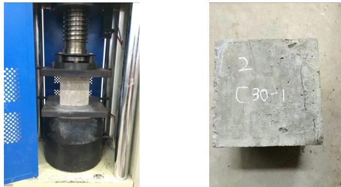
Fig. 3. Compressive strength tests of concrete
