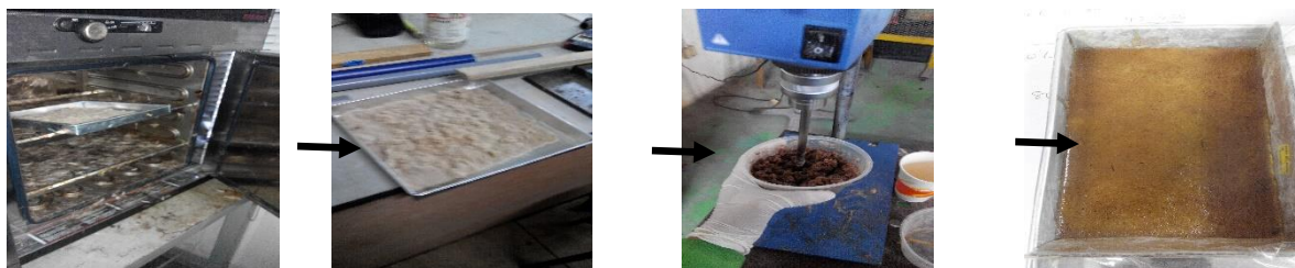
Fig. 2. Preparation of roselle fibre reinforced vinyl ester composites; a) fibre heated in the oven; b) fibre preparation; c) mix of resin and fibre; d) mixed composites poured in the mould
