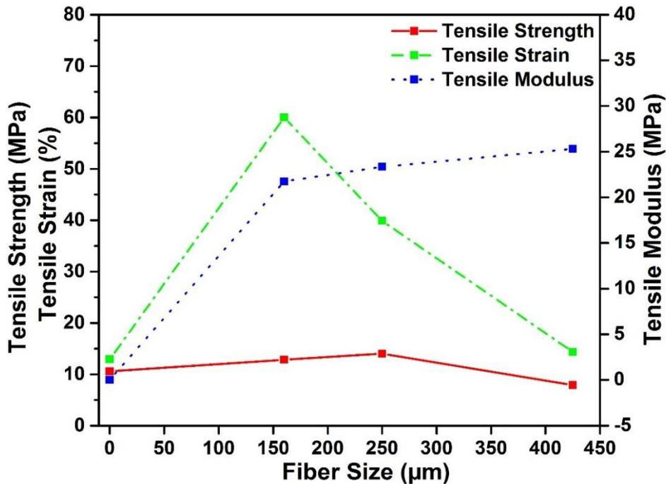
Fig. 4. Effects of the fiber size on the tensile strength, modulus, and strain of TPU-SPF composites
