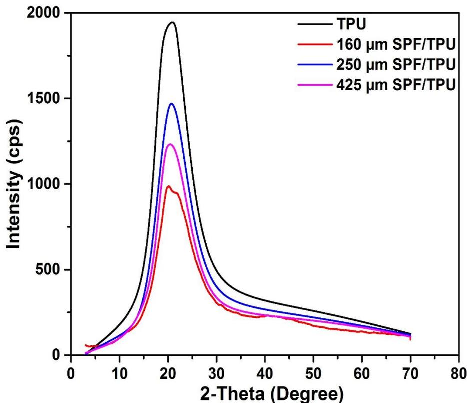
Fig. 8. XRD of pure TPU and TPU-SPF composites
