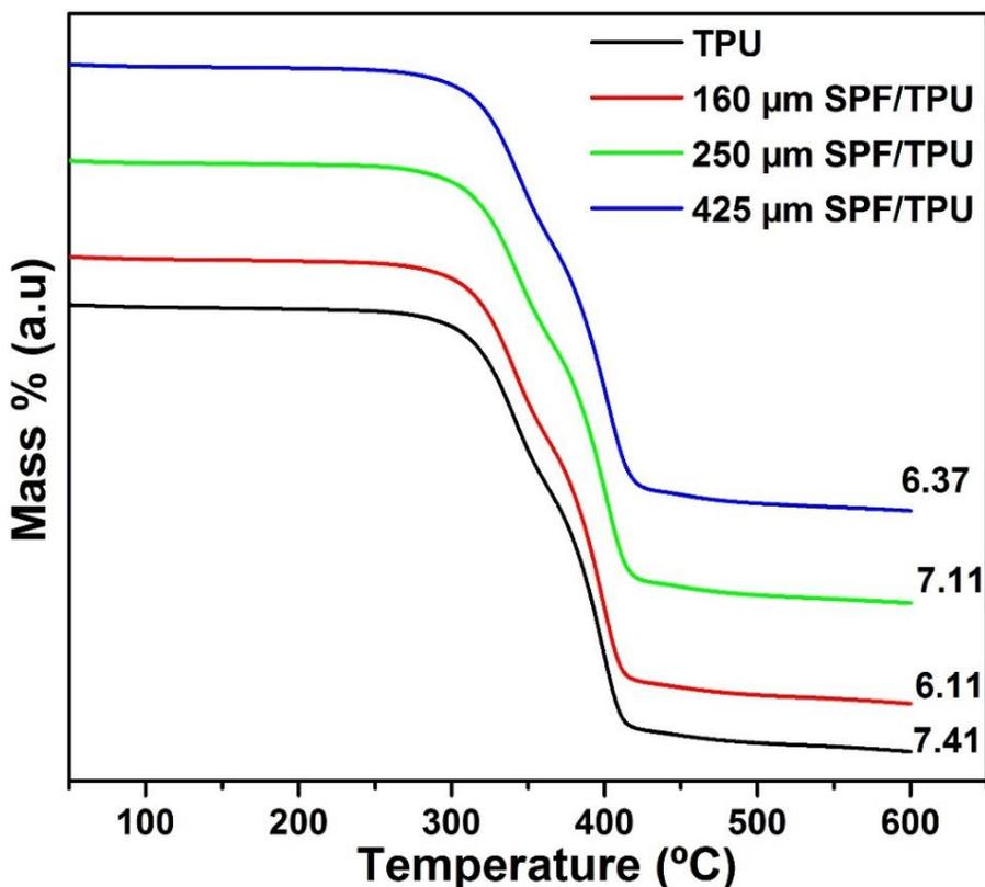
Fig. 10. TGA of pure TPU and TPU-SPF composites
