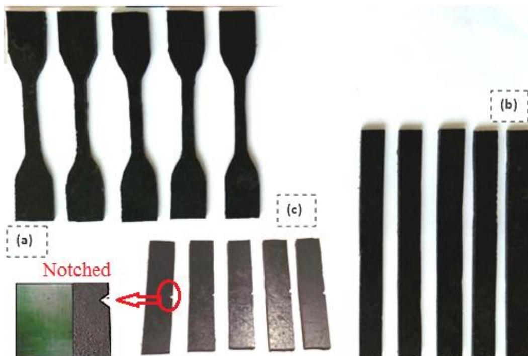
Fig. 1. (a) Tensile specimens, (b) flexural specimens, and (c) impact specimens
