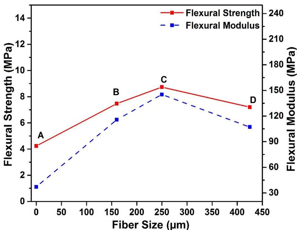
**Fig. 5.** Effects of the fiber size on flexural properties. (A) TPU; (B, C, and D) TPU-SPF composites
