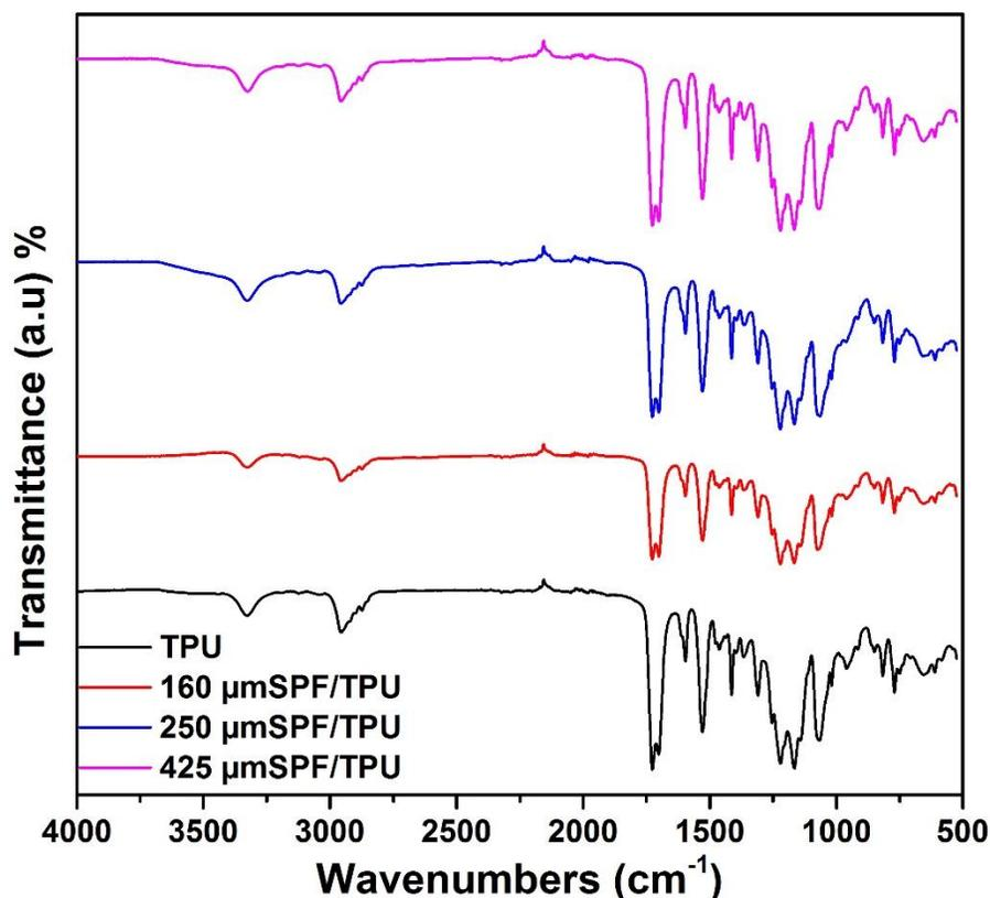
Fig. 7. FTIR of pure TPU and TPU-SPF composites
