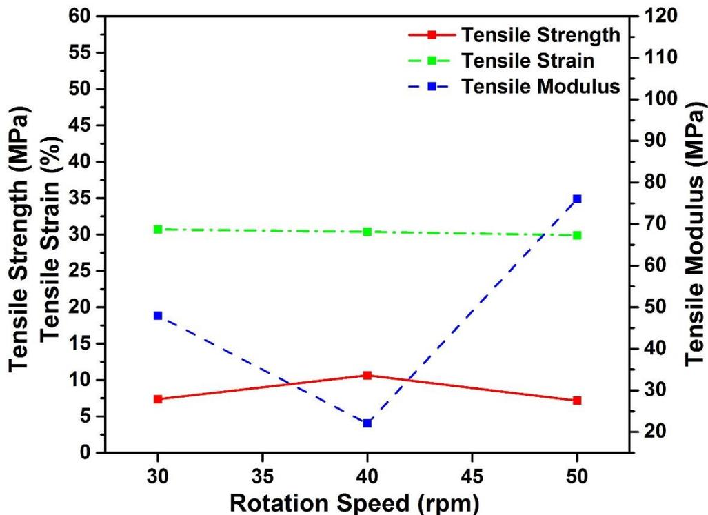
**Fig. 2.** Effects of the setting velocity on the tensile strength, modulus, and strain of TPU-SPF composites
