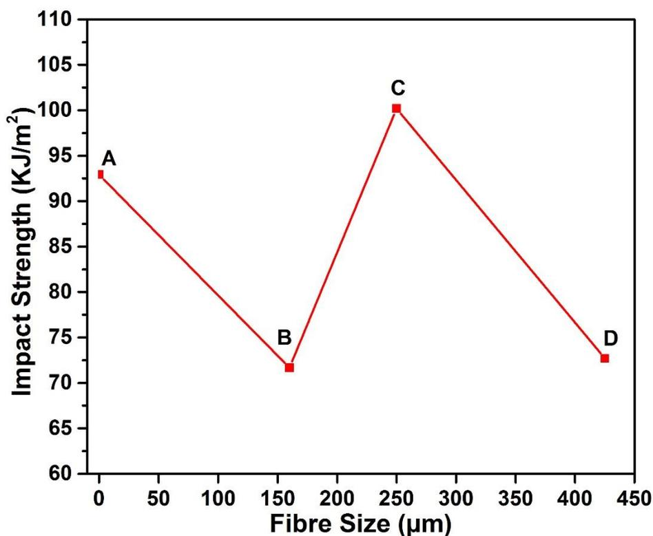
Fig. 6. Effects of the fiber size on the impact strength; (A) TPU; (B, C, and D) TPU-SPF composites
