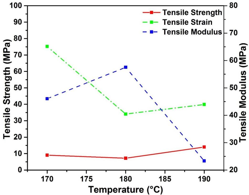
Fig. 3. Effects of setting temperature (transition phase) on the tensile properties of the TPU-SPF composites
