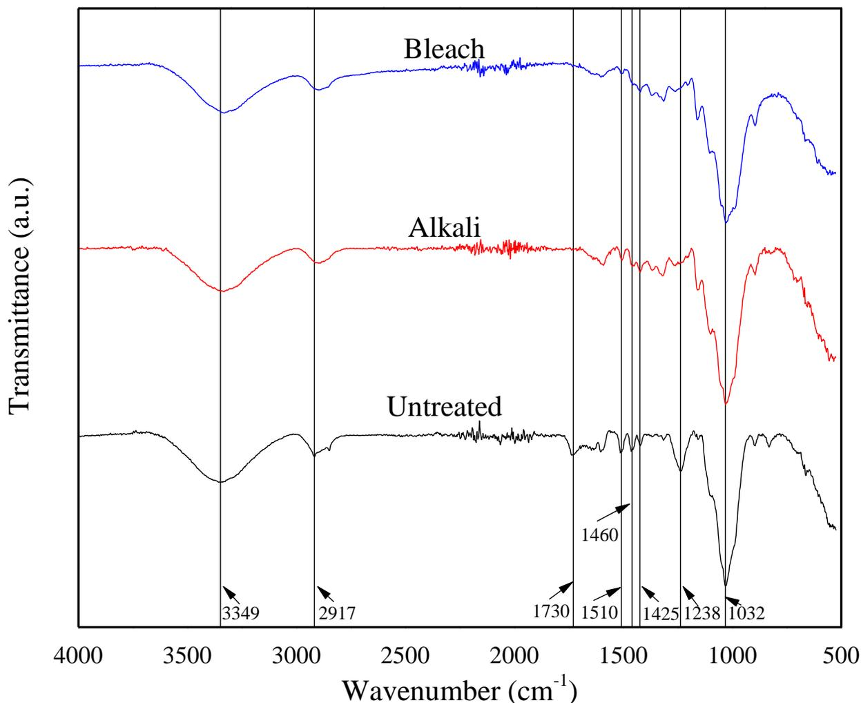
Fig. 6. FTIR spectra of untreated and treated switchgrass
