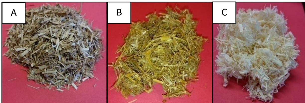
**Fig. 1.** Images of A) untreated switchgrass, B) alkali-treated switchgrass, and C) peroxide bleached switchgrass
