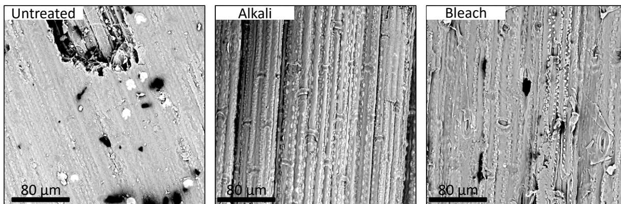
**Fig. 8.** SEM images of the surface morphologies of untreated and treated switchgrass
