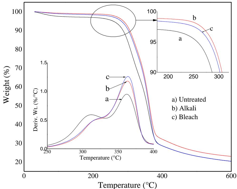
**Fig. 7.** TGA and DTG graphs of untreated and treated switchgrass
