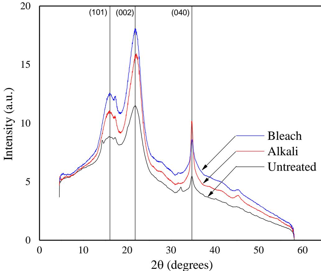
Fig. 9. XRD spectra of untreated and treated switchgrass
