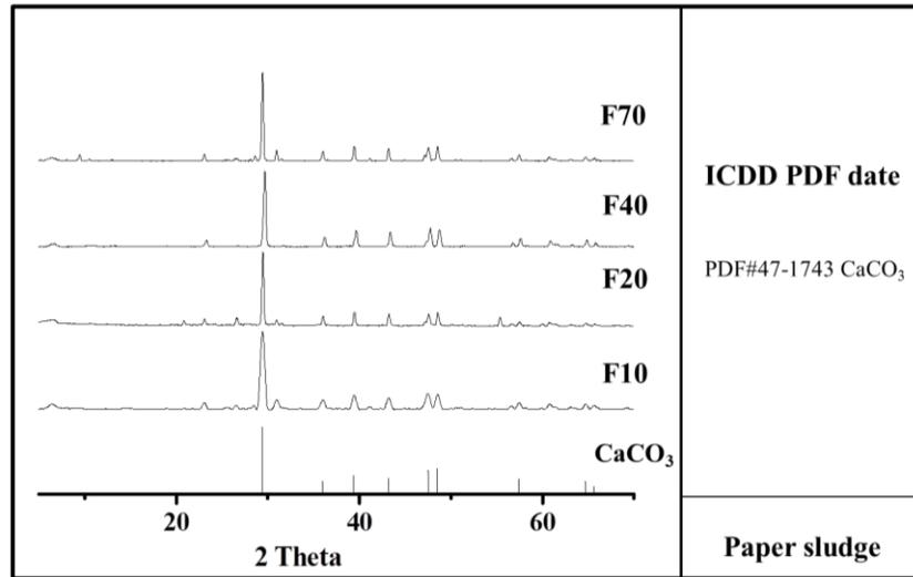
**Fig. 3.** X-ray diffraction pattern of paper sludge with different fiber contents
