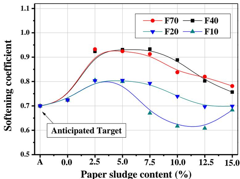
Fig. 13. Effect of paper sludge with different fiber contents on the softening coefficient of CEP mortar
