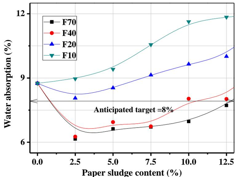
Fig. 11. Effect of paper sludge content on the water absorption of CEP mortar
