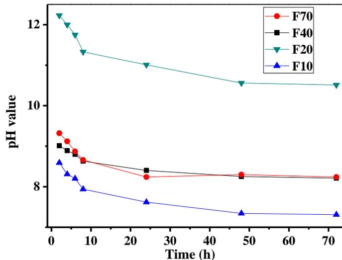
Fig. 5. Variation of the pH value of paper sludge over time
