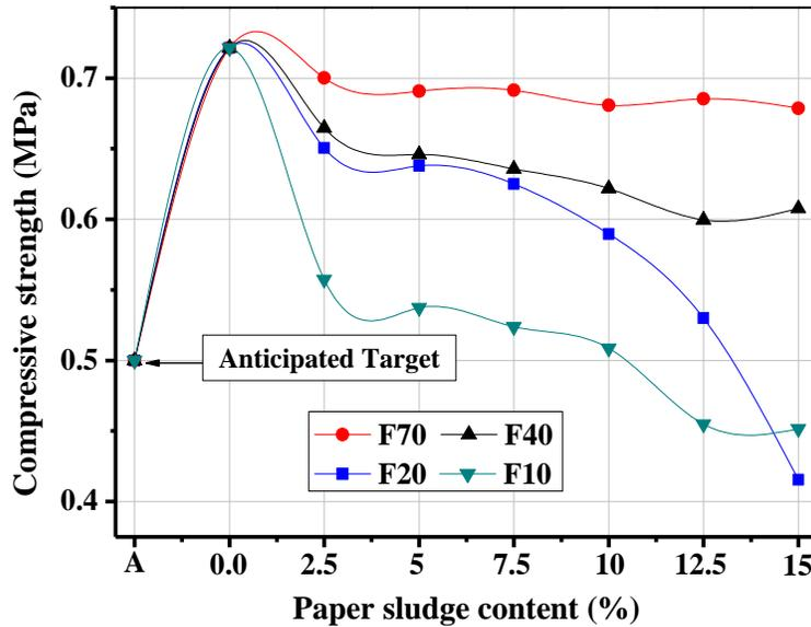
**Fig. 8.** The effect of paper sludge with different fiber contents on the compressive strength of CEP mortar
