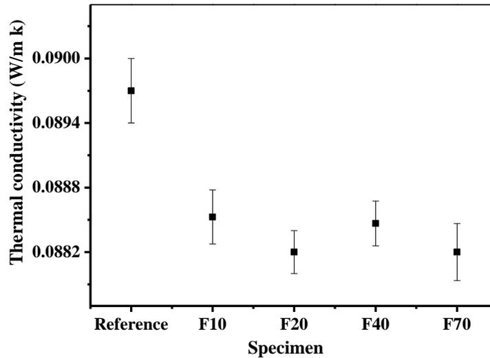
Fig. 12. Effect of 7.5% paper sludge content on the thermal conductivity of CEP mortar
