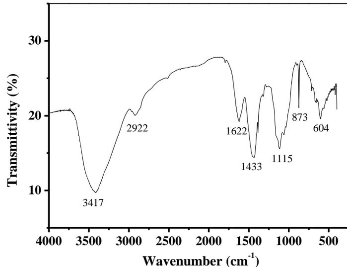
Fig. 4. Infrared spectra of wood fiber in paper sludge
