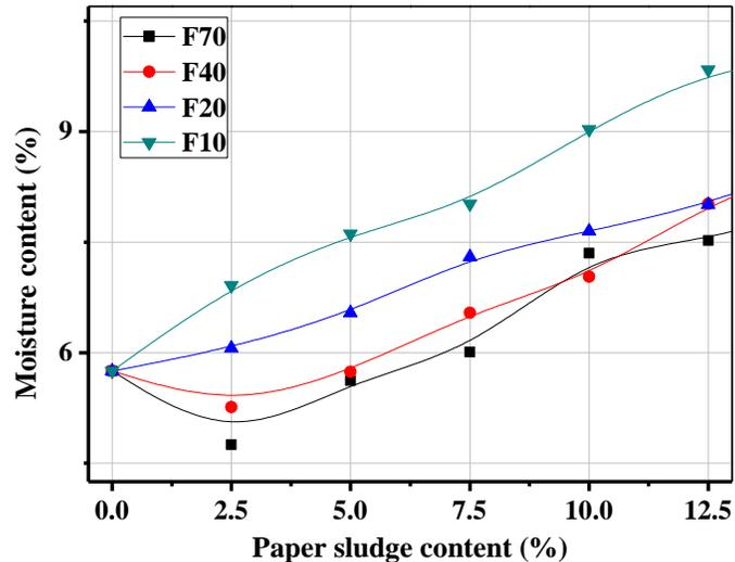
Fig. 7. Effect of paper sludge content on the moisture content of CEP mortar
