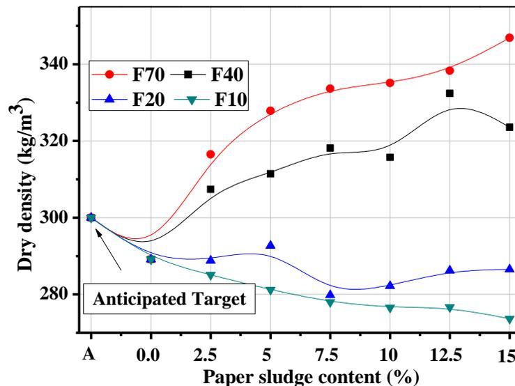
**Fig. 10.** Effect of paper sludge content on the dry density of CEP mortar
