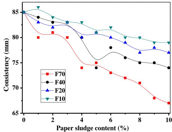
Fig. 6. Effect of paper sludge content on the consistency of CEP mortar
