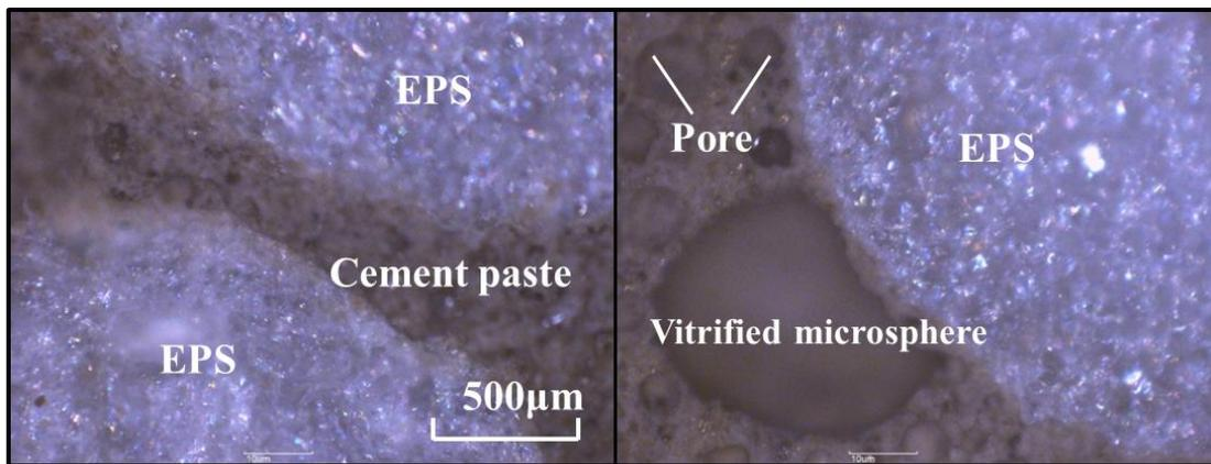
**Fig. 1.** The interface morphology of insulation mortar between EPS and the cement paste
